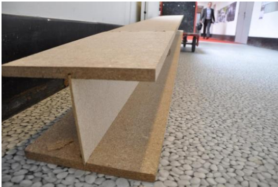
Figure 4.18, prototype with straw board and contact glue.
