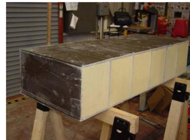
Figure 4.4, Section of a bio-composite roof source: M.A. Dweib et al., Composite Structures 74 (2006) p.37
