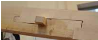
Figure 4.32, A scale 1:2 prototype of the hinge connection showed that it is a very stiff connection.
