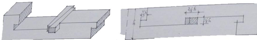
Figure 4.8, squire splice joint
