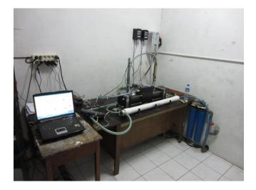
Figure 7.7: The white 2540 RO membrane is located in the front of the picture
