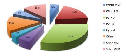
Figure 4.9: Distribution of renewable powered desalination technologies. (Data from (Eltawil et al., 2009)).
