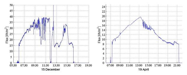
Figure 9.32: Permeate fluxes for two arbitrary days during test period 1 and test period 2 (left and right respectively).
