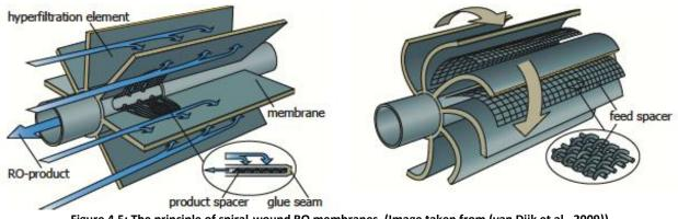
Figure 4.5: The principle of spiral-wound RO membranes. (Image taken from (van Dijk et al., 2009))
