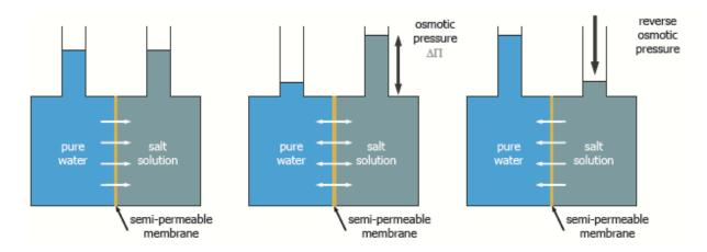
Figure 4.4: The principle of Osmosis and Reverse Osmosis. (Taken from (van Dijk et al., 2009)).
