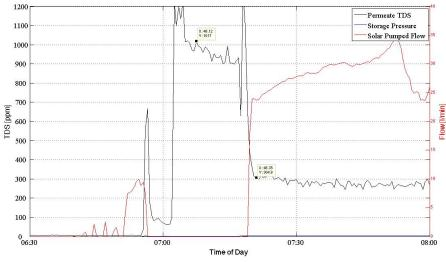
Figure 9.28: Permeate TDS during start-up on April 19th.
