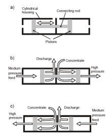
Figure 5.4: Schematic of the working principle of the Clark Pump
