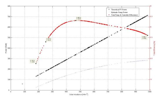
Figure 10.1: Total system efficiency, Hydraulic Power and Theoretical Power plotted versus the Solar Irradiance.
