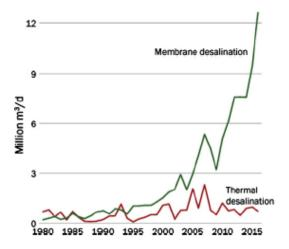
Figure 4.10: Comparison between membrane desalination capacity and thermal desalination capacity from 1980 to 2016. (Taken from (Misdan, Lau, & Ismail, 2012)).
