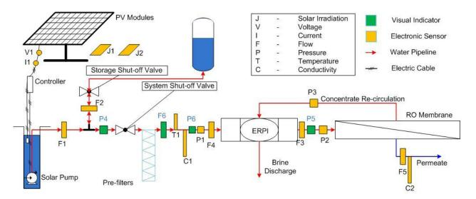
Figure 7.10: Sensors & visual indicators integrated into the system
