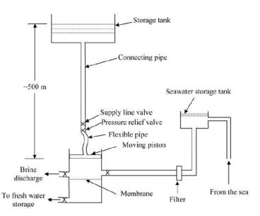
Figure 4.12: Proposed hydrostatic desalination installation. (From (Al-Kharabsheh, 2006)).
