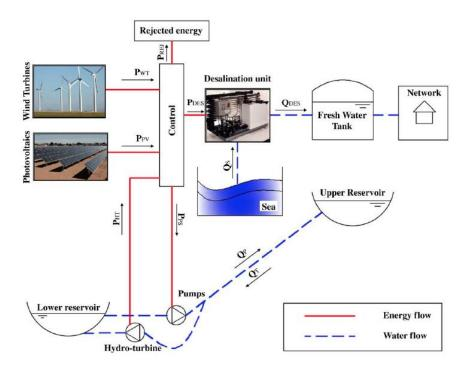
Figure 4.13: Hybrid RO Desalination design, with a PSP. (Taken from (Spyrou & Anagnostopoulos, 2010)).
