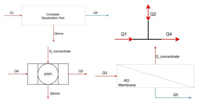
Figure 7.11: From top left corner to the bottom right corner: mass balance (MB) over the complete system, MB over T connection, MB over the ERPI, MB over the RO membrane.
