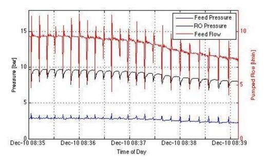
Figure 9.5: Feed pressure, RO pressure and feed flow during a 4-minute period on December 10<sup>th</sup> 2012.
