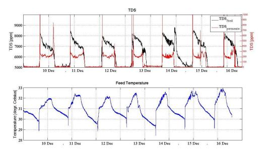
Figure 9.8: Feed and Permeate TDS on the top, and feed water temperature on the bottom.
