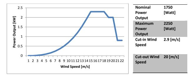
Figure 6.2: Power curve & relevant specifications for the donQi Urban 1.5 Venturi Windmill
