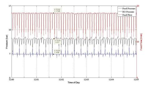
Figure 9.18: Feed- and RO pressure and feed flow during a 5 minute period on April 19th.
