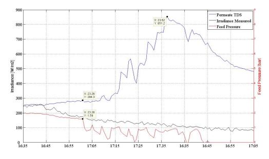
Figure 9.13: A closer look at the permeate TDS, Irradiance measured and feed pressure during shutdown.
