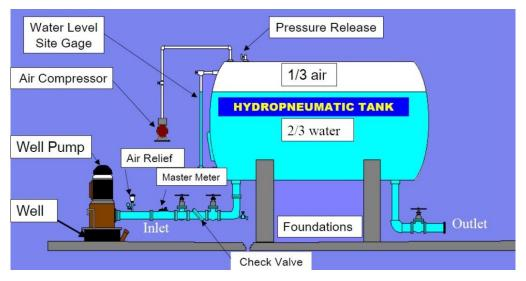
Figure 5.3: Schematic view of a typical hydro-pneumatic tank, source: (Pandolph, Unknown)
