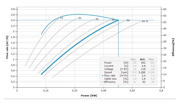
Figure 8.1: Pump Curves according to the manufacturer.
