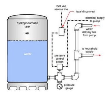
Figure 5.2: Typical hydro-pneumatic vessel, source: ("Water Safe bc," 2006)
