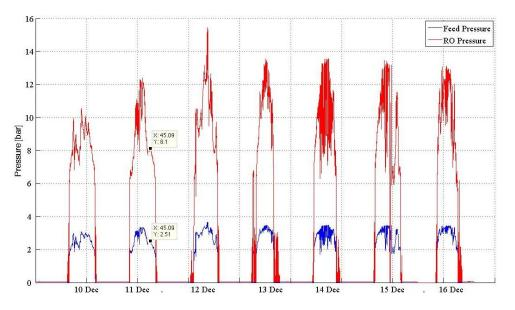
Figure 9.3: Feed and RO pressures measured during initial test run.
