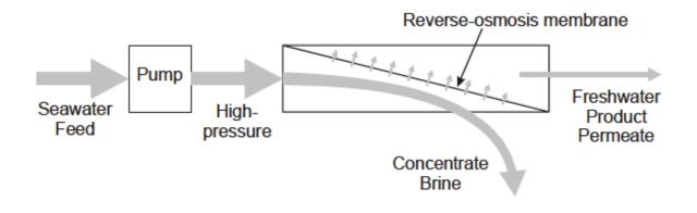
Figure 4.6: Schematic presentation of a simple RO desalination plant. (Image taken from (El-ghonemy, 2013a)).
