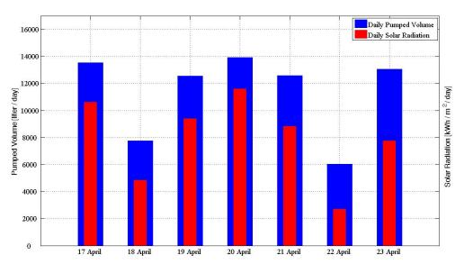
Figure 9.14: Daily solar radiation and pumped volume for second test period.
