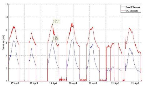
Figure 9.16: Feed- and RO pressure measured during the second test period.
