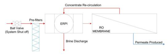
Figure 7.2: Detailed schematic of the desalination part
