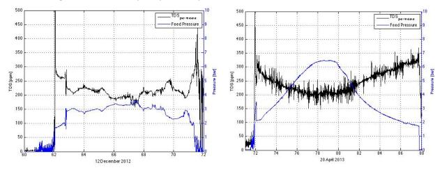
Figure 9.31: Feed pressure and permeate TDS for period 1 and period 2 (left and right respectively).
