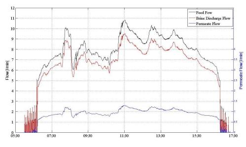
Figure 9.6: Feed flow, permeate flow and brine discharge flow for 10 December 2012.
