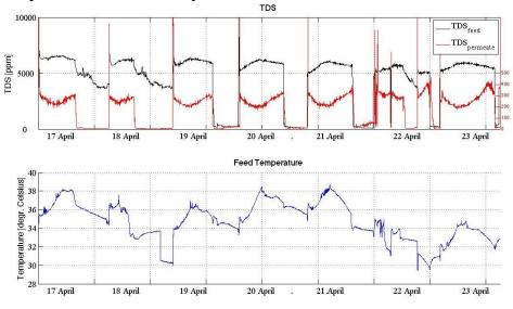
Figure 9.21: Feed- and permeate TDs at the top and feed water temperature at the bottom.
