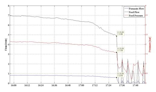
Figure 9.12: Feed flow, permeate flow and feed pressure during shut-down on December 10<sup>th</sup> 2012.
