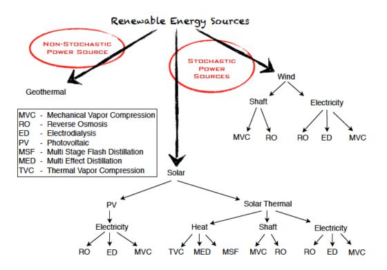
Figure 4.8: Possible configuration of renewable energy sources and desalination processes. (From (Eltawil et al., 2009) via (Thye, 2010)).
