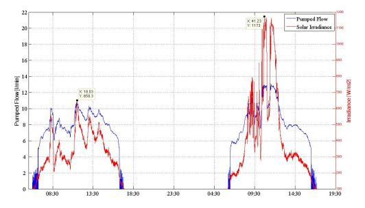
Figure 9.2: Solar Irradiance and pumped flow for 10 & 11 Dec (days 1 & 2 of test run).
