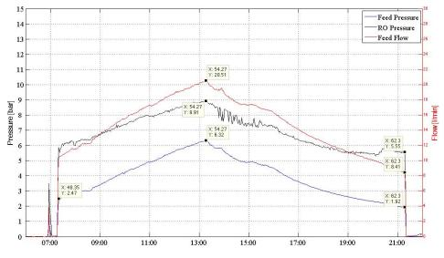
Figure 9.17: Feed pressure, RO pressure and solar pumped flow on April 19th.
