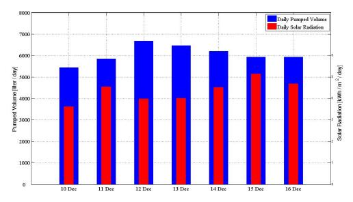
Figure 9.1: Daily solar radiation and daily pumped volume for initial test run.
