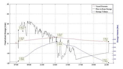
Figure 9.26: Storage pressure, volume and flow on April 19th.
