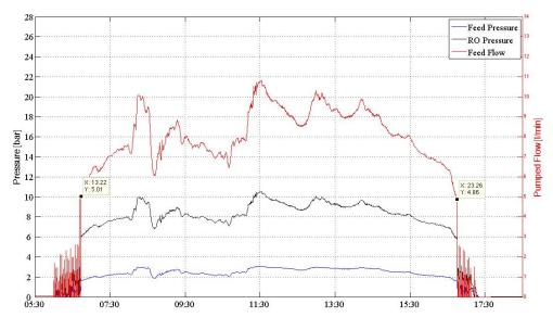
Figure 9.4: Feed pressure, RO pressure and feed flow on 10 December 2012.
