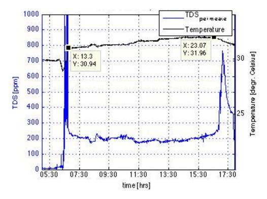
Figure 9.9: Permeate TDS and feed temperature for December 10<sup>th</sup> 20120.
