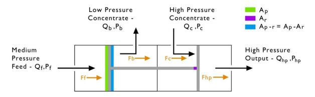
Figure 5.5: Explanation of the working forces inside the pressure intensifier.
