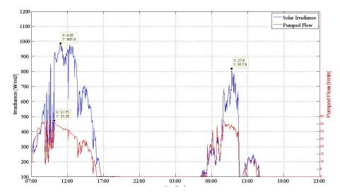
Figure 9.15: Solar irradiance and pumped flow for 17 & 18 April (Days 1 and 2 of test period).
