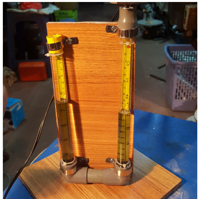
Image 3.3.2: Mono-meter for pressure measurement
