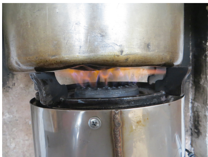
Figure 11 Flame during the simmer test
