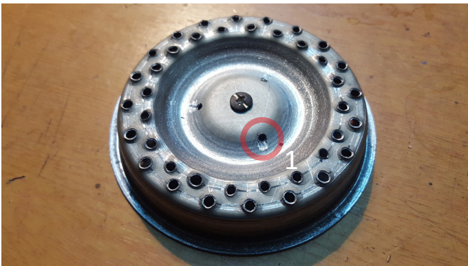
Image G.2.45: Improved burner top with center primer holes
