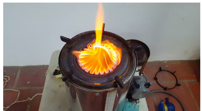
Image G.2.17: Gasifier in operation without the burner on top, creating a vortex flame
