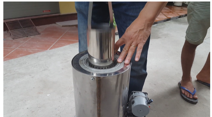
Image G.2.14: Placement of the reactor through the funnel
