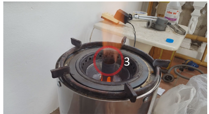
Image G.2.15: Venturi tube accelerating the gas during operation
