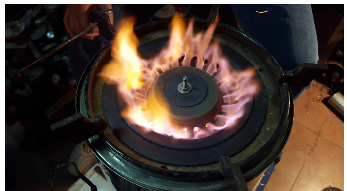
Image G.2.60: Burner placed on top of the reactor
