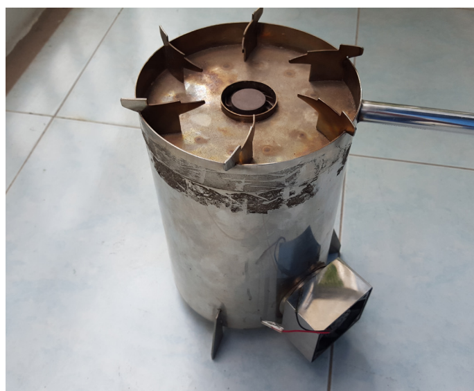
Image B.4.5: 2015 model forced primary and secondary air
