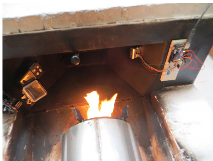
Image 8.1.2: Test setup of the stove and measuring devices
