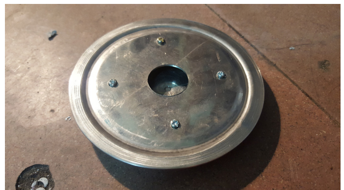
Image G.2.11: Bottom view of the burner top
