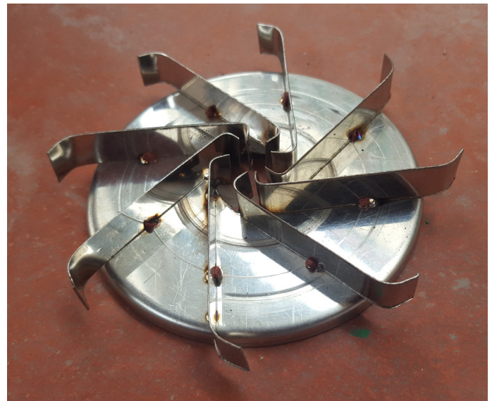
Image C.3.1: Close up of the burner mixer
