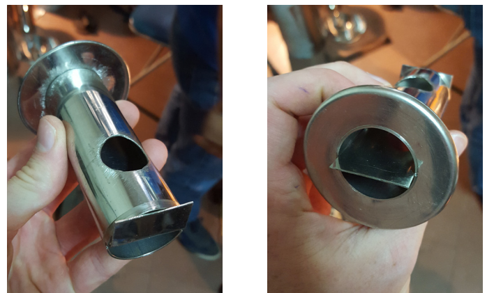
Image C.3.16: Air flow division tube for primary and secondary air
