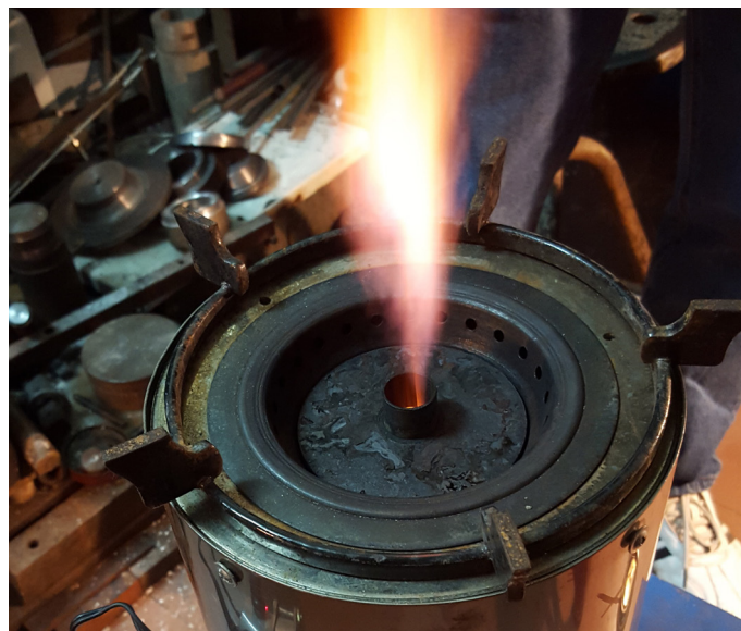
Image G.2.47: Reactor cap placed on top of the gasifier during operation
