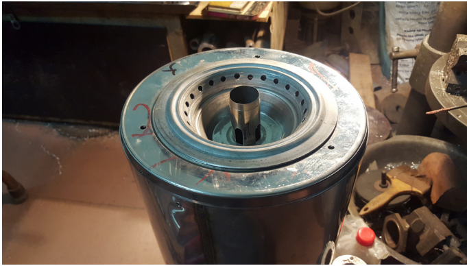
Image G.2.12: Placement of the burner cap with venturi tube
