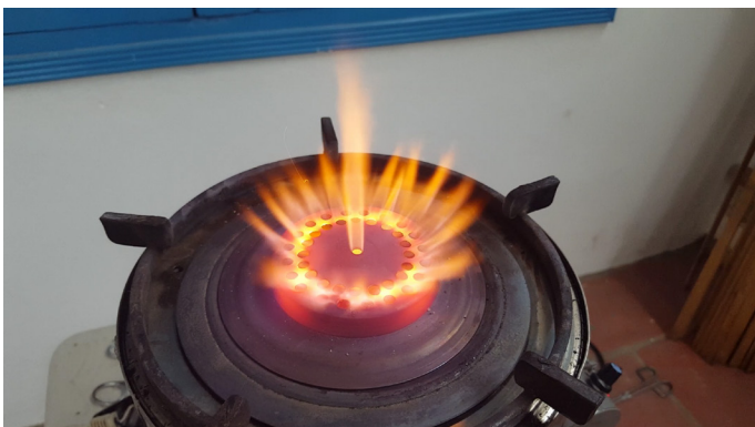
Image G.2.16: Burner placed on top getting red hot
