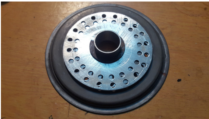
Image G.2.43 & G.2.44: Boundary plates showing different positions of the added ring to adjust the airflow of the secondary air.
