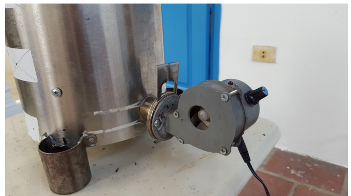
Image C.3.15: Close up image of the centrifugal fan attached to the gasifier with control valves
