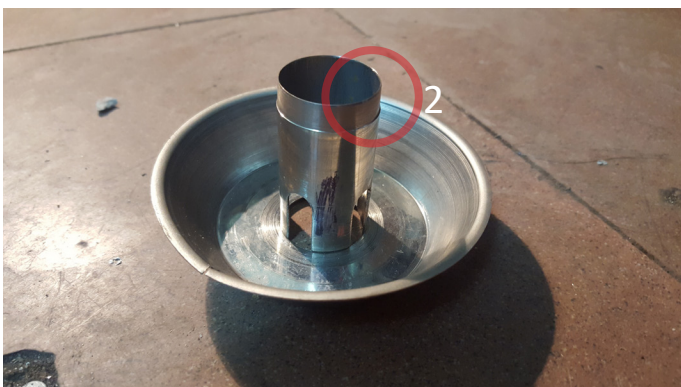
Image G.2.10: Burner cover with venturi tube
