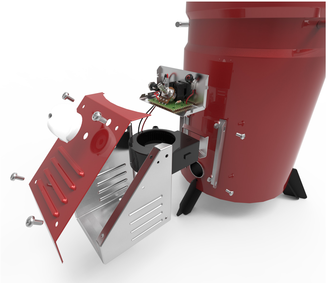
Image 6.12.5: Exploded view of the electronic storage box
