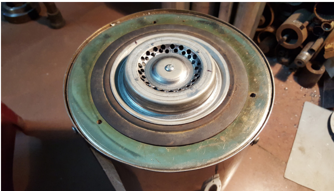
Image G.2.28: Incline burner placed on the gasifier
