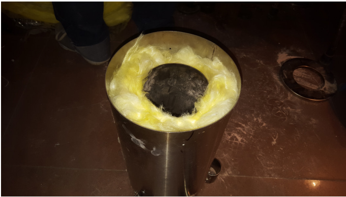
Image 6.7.1: Filling the outer body of the prototype with glass fiberglass insulation
