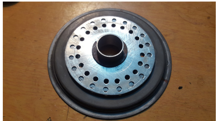
Image G.2.43 & G.2.44: Boundary plates showing different positions of the added ring to adjust the airflow of the secondary air.
