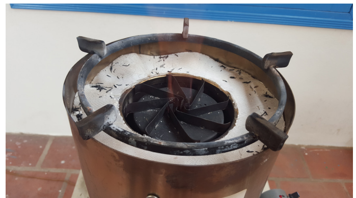
Image C.3.5: Close up of the pot support ring
