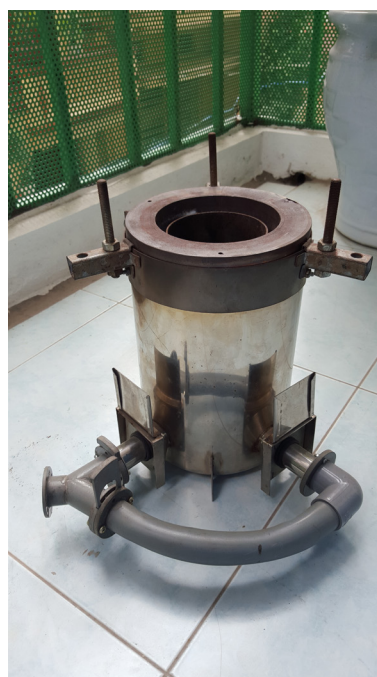
Image B.4.6: improved 2015 model with separate control for the secondary air
