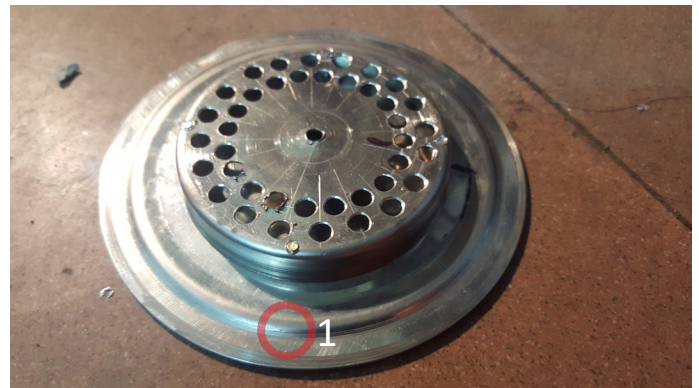
Image G.2.9: Top view of the burner top with two circular patterns rows 20 holes
