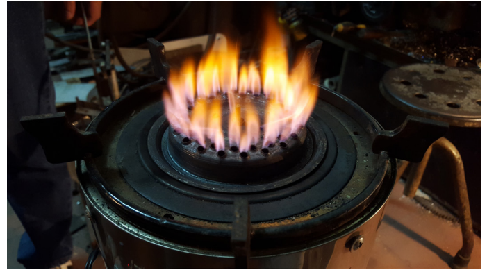
Image 6.4.3: Produced flame burning on top of the burner ports
