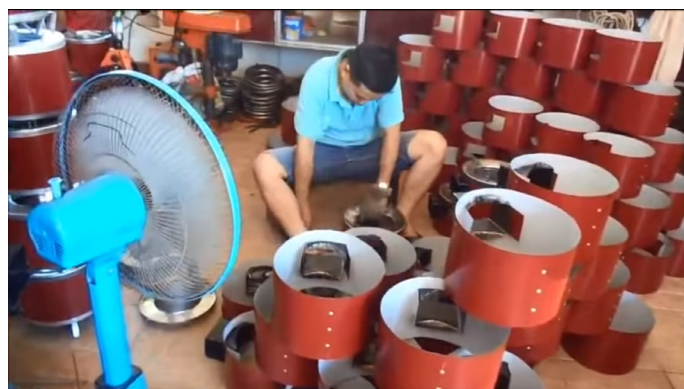
Image H.5.1: Solarserve stove production line in Vietnam showing different stages in the manufacturing and assembly process. (YouTube, 2014)
