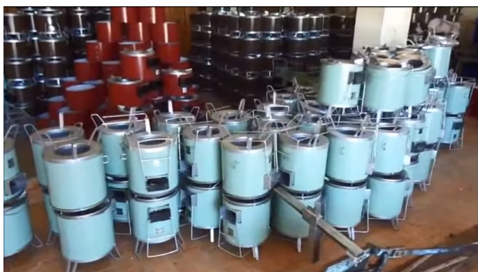
Image H.5.1: Solarserve stove production line in Vietnam showing different stages in the manufacturing and assembly process. (YouTube, 2014)
