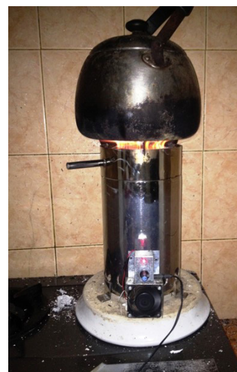
Image B.4.4: 2014 version forced primary air, draft secondary air
