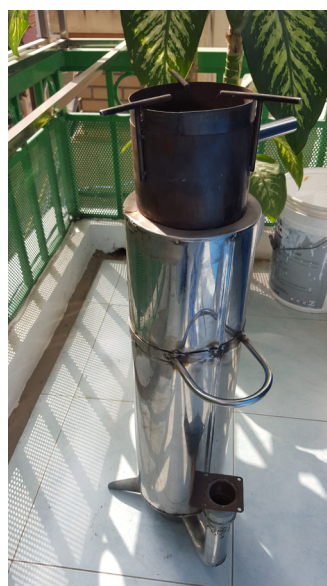
Image B.4.2: 2012 rice husk gasifier based on Belonio's design
