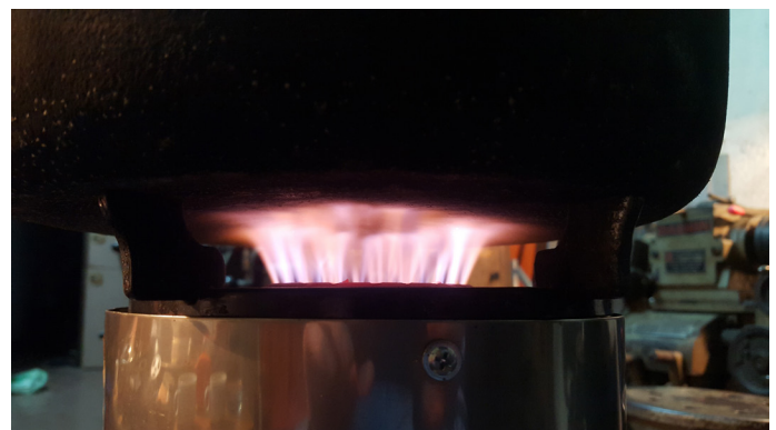
Image G.2.32: Flame of the flat burner in high power mode with a pot placed on top
