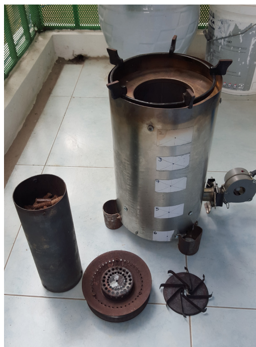
Image B.4.7: 2015 model gasifier with improved burner and airflow control
