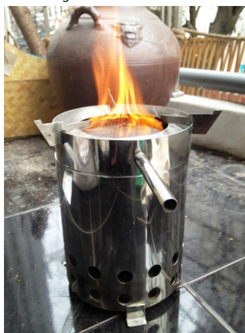
Image B.4.3: 2013 natural draft pellet gasifier
