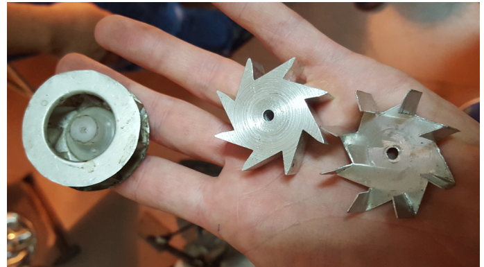
Image C.3.14: Molds for centrifugal fan blades.
