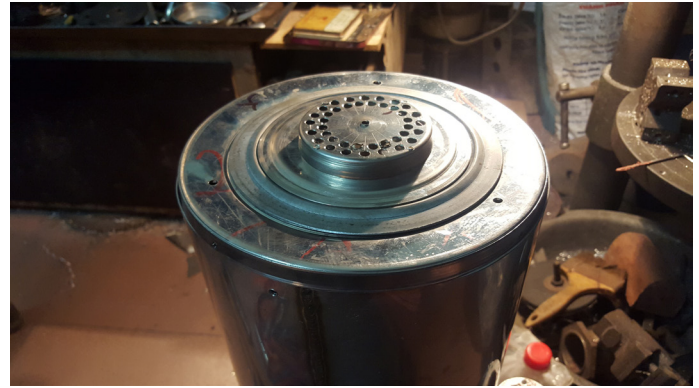
Image G.2.13: Placement of the burner on top of the gasifier
