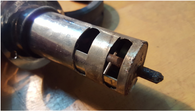
Image 6.3.2: Close-up of the two air slots
