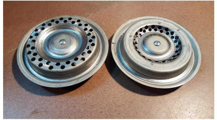
Image G.2.26: Top view of the two prototype burners
