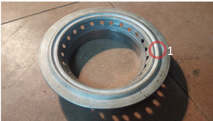
Image G.2.8: The funnel with holes drilled on the side
