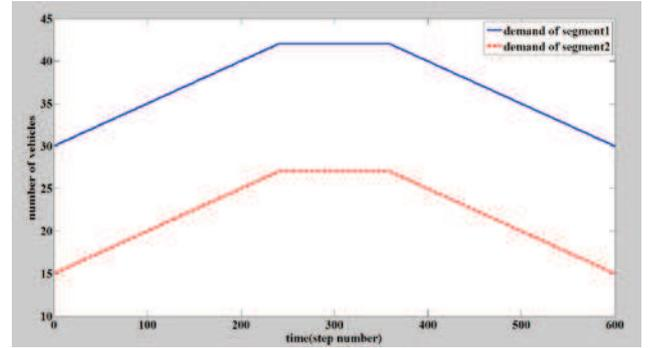
Fig. 4. Demand of origin 1 and 2. The peak demand of cell 1 is 42veh/step and cell 2 is 27veh/step.
