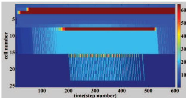
Fig. 6. Traffic density of every cell without traffic control when disturbance happens
