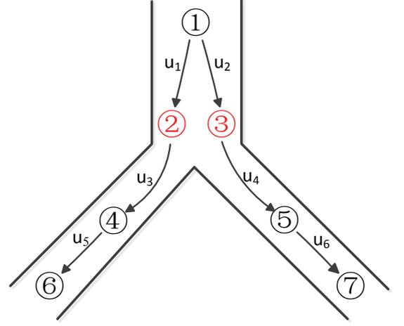
Fig. 1. Description of cells and links of a network. Red cells are decision cells.
