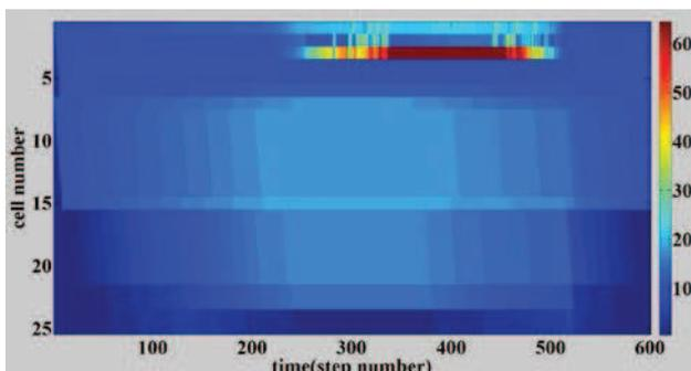
Fig. 7. Traffic density of every cell with traffic control when disturbance happens
