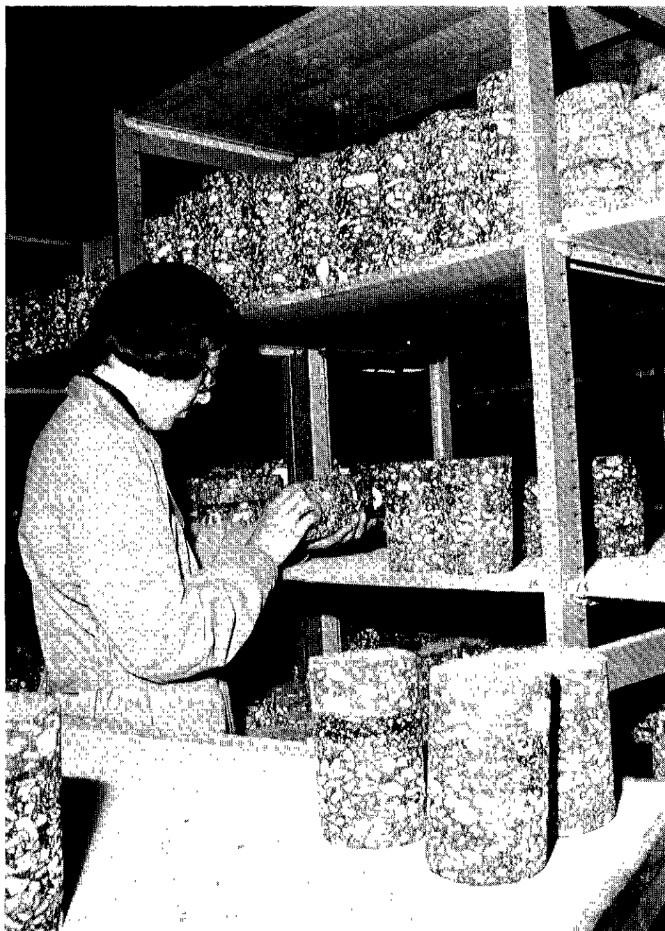
Figure 1. Cores, drilled out of the pavement, intended for testing in relation to acceptance control of pavements.
