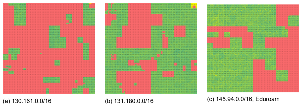
Figure 6.2: The Hilbert visualization of the three available ranges. The number of connections are mapped to a color gradient from red to green. Red indicates no connections, green indicate the highest number of connections.
