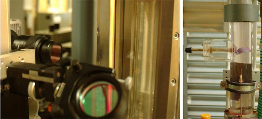
(a) High-Speed camera (left) and the conical pipe of the (b) Bubble injector with measurement section (right); the mirror in the front is the needle and the turnable spoon ( $V=2\text{cm}^3$ )
