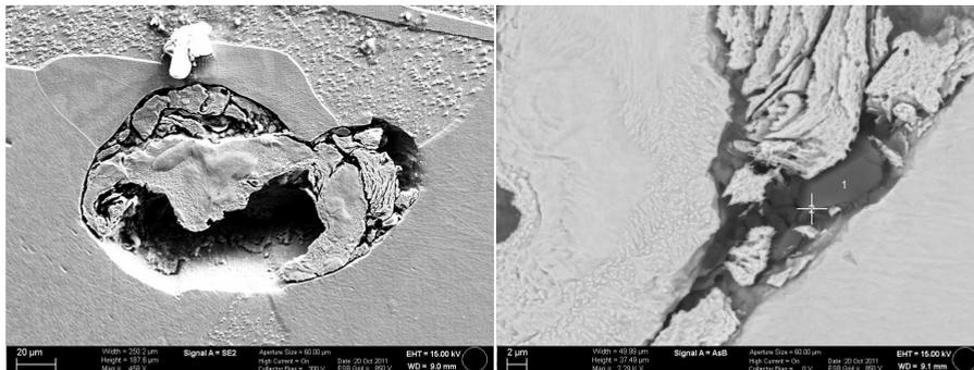
(c) Cavity from an Argon bubble with inclusions (dark grey), the light grey areas in the cavity are not inclusions but the remains of oxidised steel during sample preparation
