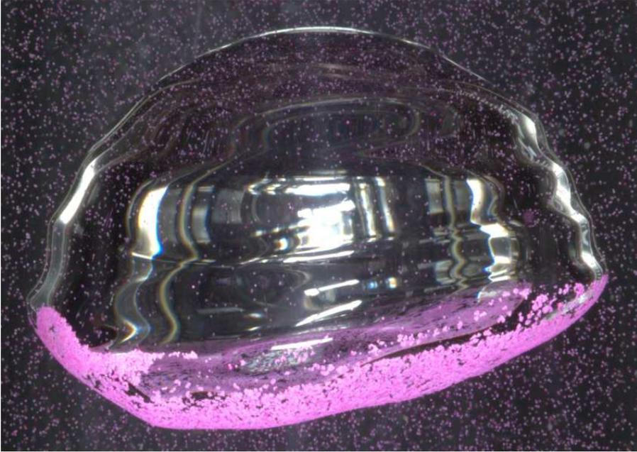
Figure 5.15: Bias in the particle counting leading to the observed maximum in Fig. 5.14: Together with the pink particles detected at the bottom of the bubble, also the inner side of the bottom can be observed by refraction
