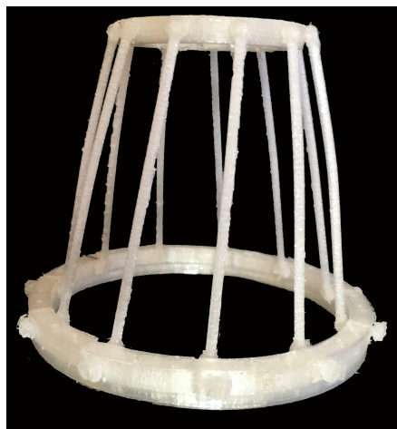
(b) Image half-mast showing plastic deformation after buckling
