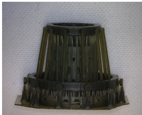
Figure 5.24: EnvisionTEC mast with support material.
