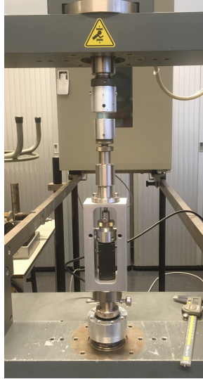
Figure 4.13: Test setup tension/torsion bench at department of Presesion and Microsystems TUDelft.
