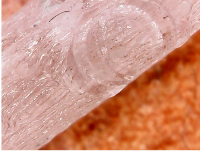
Figure E.11: This figure shows specimen deformation and slip of attachment point of the mounting apparatus of the Zwick prototype machine, used for torsion, tension, and compression.
