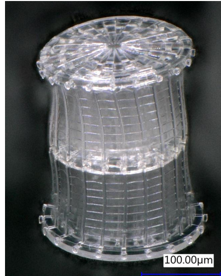
(b) Double stack mast printed on Nano-scribe.
