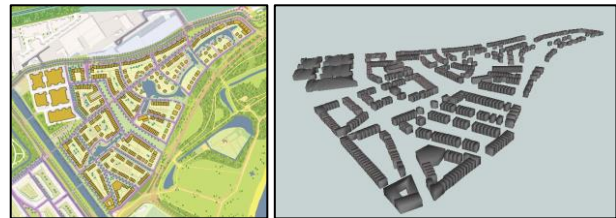
Figure 7. [Left] In orange, the manually digitized building footprints, shown on top of the georeferenced "Nieuw Kralingen" plan. Image adapted by the authors and originally from: architectuur MAKEN (n.d.). [Right] Resulting 3D model of "Nieuw Kralingen" visualised in FME Data Inspector.
