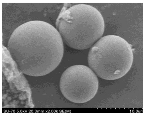
Figure 5: the SEM picture of E-51/UF microcapsules synthesized in optimal process
