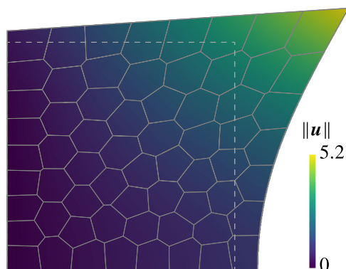
Fig. 5. Deformed configuration for the high-order patch test, showing in colors the magnitude of the displacement field.
