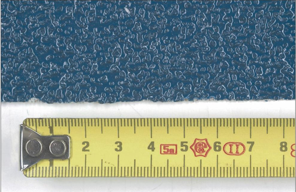
**Appendix 68 Photographs of OD 200 mm pipe with 500 micron sand roughness**
