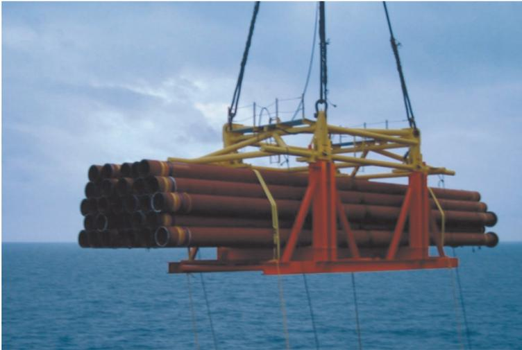
Figure 2-4 Riser pipes (double joints).
