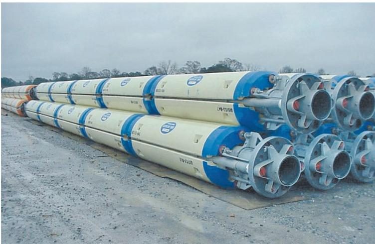
Figure 2-5 Offshore drilling riser with buoyancy modules.
