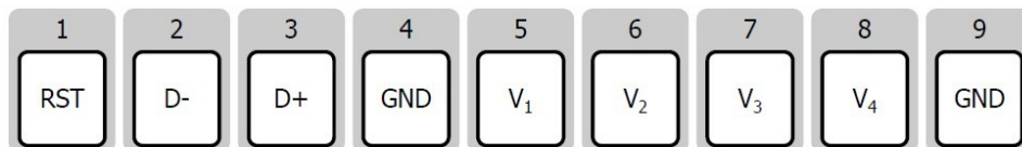
Figure 2. PQ9 connector form factor on Delfi-PQ PCB 2
