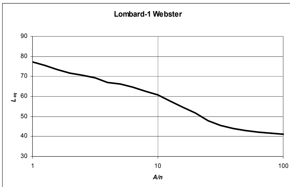
Figure 44. Equivalent sound level (Group vocal output) as a function of the amount of sound absorption per capita (Webster).
