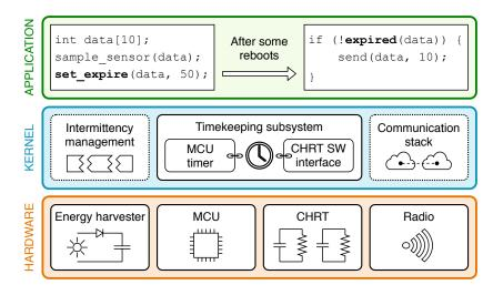
Figure 4.1: Botoks high-level architecture. The runtime kernel keeps track of time using the CHRT. Applications are instrumented with CHRT functions to infer on the elapsed time despite power outages.
