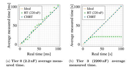
Figure 6.1: CHRT average measured time for time measurements in the intervals 1 ms to 100 ms (tier 0, resolution of 1 ms) and 1 s to 100 s (tier 3, resolution of 1 s).
