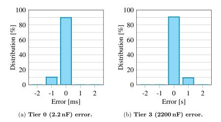
Figure 6.2: CHRT error distribution for time measurements in the intervals 1 ms to 100 ms (tier 0, resolution of 1 ms) and 1 s to 100 s (tier 3, resolution of 1 s).
