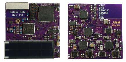
Figure 5.1: Botoks platform. The front (left) contains radio, antenna, solar panel and MCU. On the back side (right) is the Cascaded Hierarchical Remanence Timekeeper. The board dimensions are  $1^{"}\times1^{"}$ .
