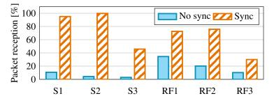
Figure 6.5: Percentage of received packets for a point-to-point link between two Botoks devices, measured in six different energy harvesting conditions described in Table 6.2. The percentage of packets received using the CHRT-powered synchronization algorithm is compared to the baseline case—with no synchronization. Note that for S3 and RF3 the maximum packet reception available is 50%, as the receiving node does not have enough energy to wake up as fast as the transmitting node.
