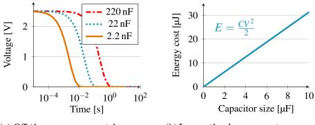
(a) Off time measurement increases with capacitance.
