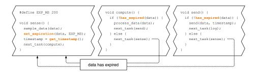
Figure 5.3: Example usage of the high-level CHRT API. The program is a typical sensing routine, and the API is used to specify that the elapsed time between sensing and transmission of some data must not exceed 200 ms of absolute time (on and off), as well as to get a timestamp to be sent together with the data.
