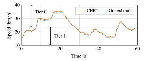
Figure 6.4: Calculated speed of the bicycle, in km/h, over a period of 60 s. The result obtained with Botoks and its embedded CHRT is compared to the ground truth. As shown, the two smallest tiers of the CHRT are dynamically used through the experiment.
