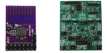
Figure 5.2: Botoks hardware modules, including distinct development platforms for working with the CHRT (right), and ultra-low-power radio (left). These hardware options provide multiple ways to integrate timekeeping into emerging battery-less applications.
