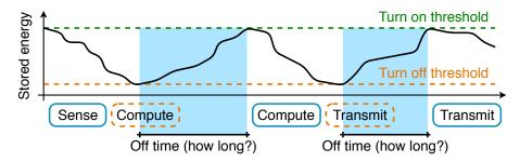
Figure 1.1: Energy-harvesting battery-less sensors operate intermittently, with execution broken up by power failures of unpredictable duration. These off times are hard to measure with existing timekeepers such as real-time clocks.
