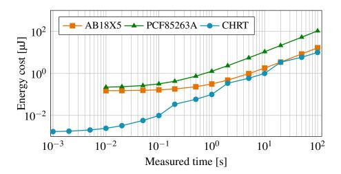
Figure 6.3: Comparison between CHRT and two RTCs from Table 3.1 of the total energy required to time a period. The CHRT allows for millisecond timing whilst requiring less or similar energy compared to the lowest power RTC.
