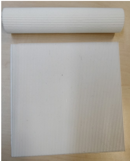
(a) 3D printed mould used for making the fins
