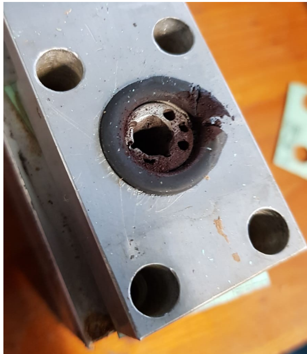
Figure H.1: Corrosion in the flow channels of the aluminium block.
