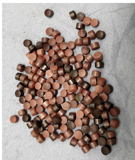
Figure 3.6: Catalyst pellets as sourced from the manufacturer (The red colour of some of the pellets is due to prior reduction with H 2 ).
