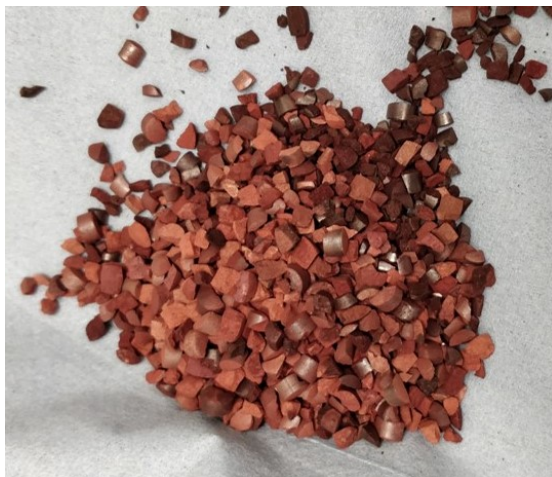
Figure 4.18: 5 mm catalyst pellets cut into two halves along the central axis.
