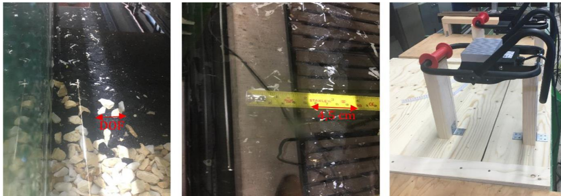
Figure 30 - FOV with black stones and DOF (left), DOF (middle) and setup of LED lights (right) (Kramer, 2016)
