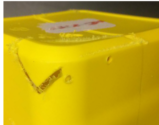
Figure 5.90: second test - Real environment with curve and holes out of position
