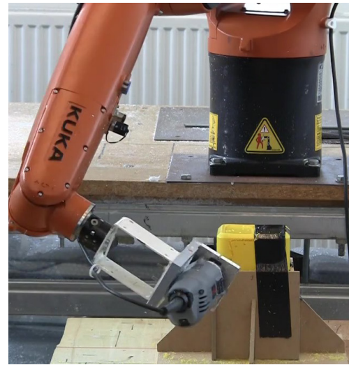
STEP 1 : CUTTING LATERAL COMPONENTS
