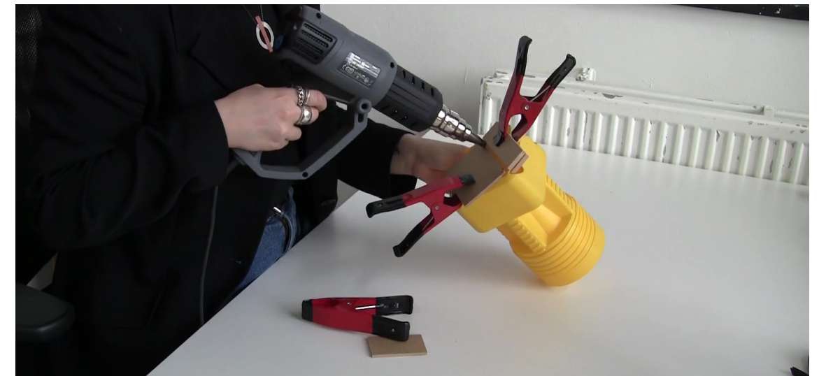
Figure 5.98: third test - STEP 2 | folding parts with an heat gun
