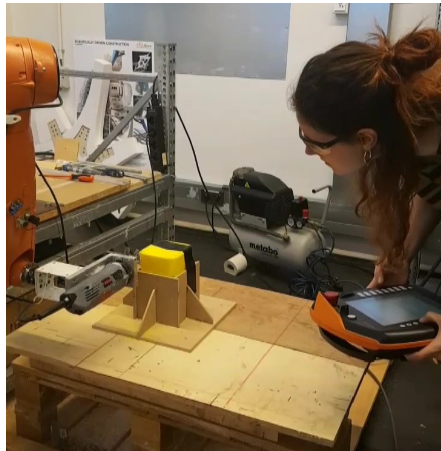
Figure 5.97: third test - STEP 1 | drilling holes & material removal
