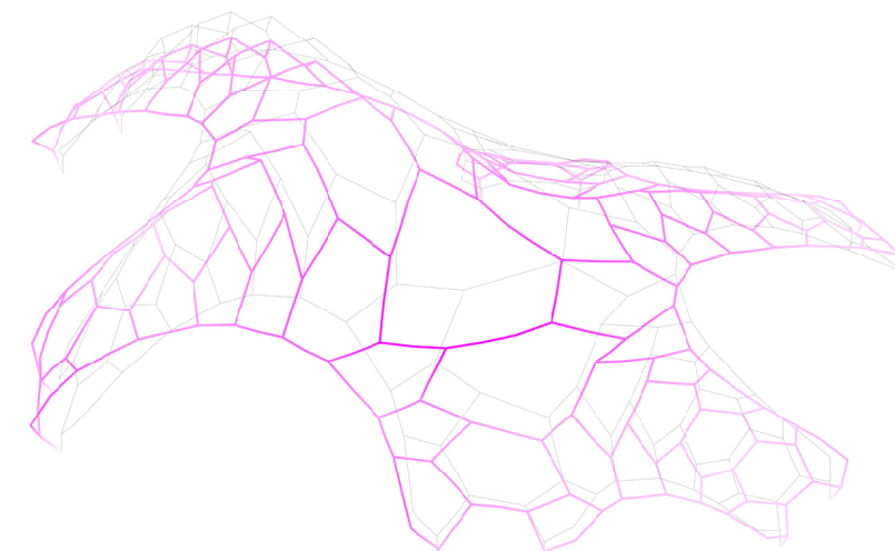
Figure 5.138: Karamba - maximum deformation of the structure (PE)
