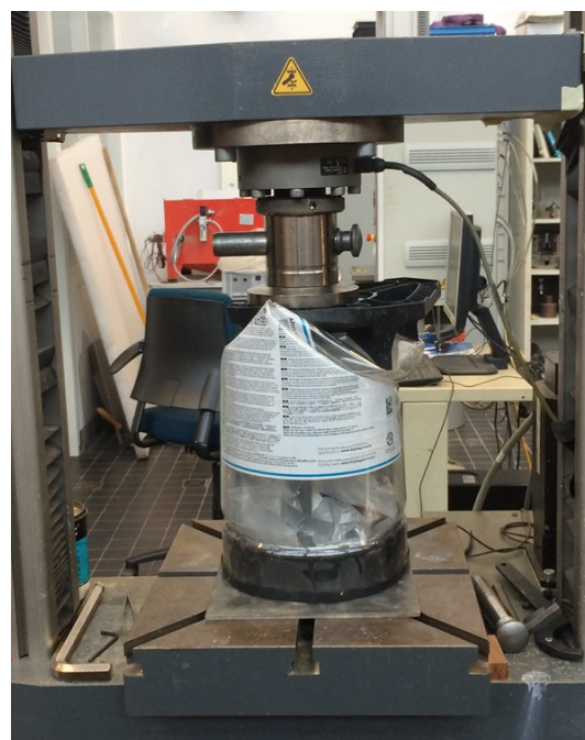
Figure 5.32: disposable keg I test 2
