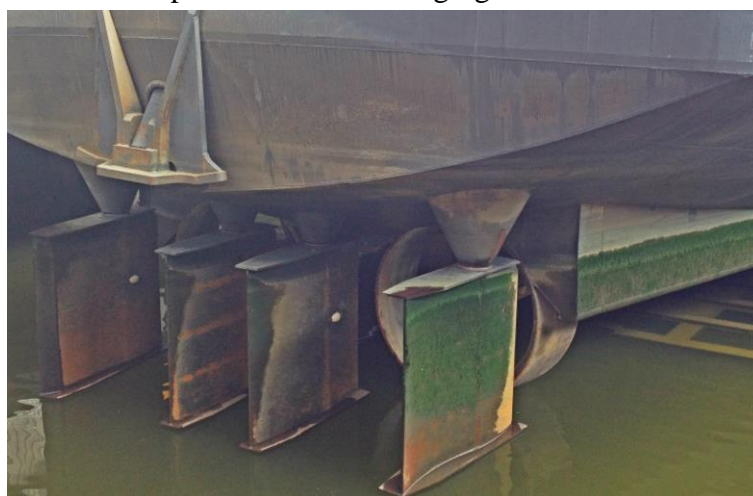
Fig. 3 An inland vessel equipped with 4 rudders and twin propeller Characteristics of inland vessel configurations are compared to those of sea-going ships in this section. Among the differences are higher block coefficients, larger width
