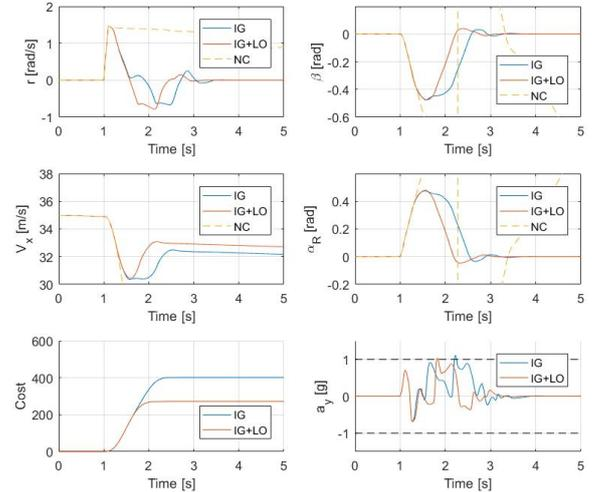
Fig. 9. Vehicle states according to simulation with an initial speed of 126 km/h. The lateral impact was exerted at  $T=1.0$ s. NC for no control, IG for controlling with initial guess and IG+LO for controlling with NMPC.
