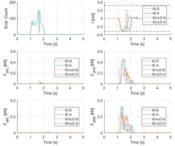
Fig. 8. Controller's action according to simulation with an initial speed of 50 km/h. The lateral impact was exerted at  $T=1.0$ s. NC for no control, IG for controlling with initial guess and IG+LO for controlling with NMPC. D for control demand and A for actual response of the actuators.
