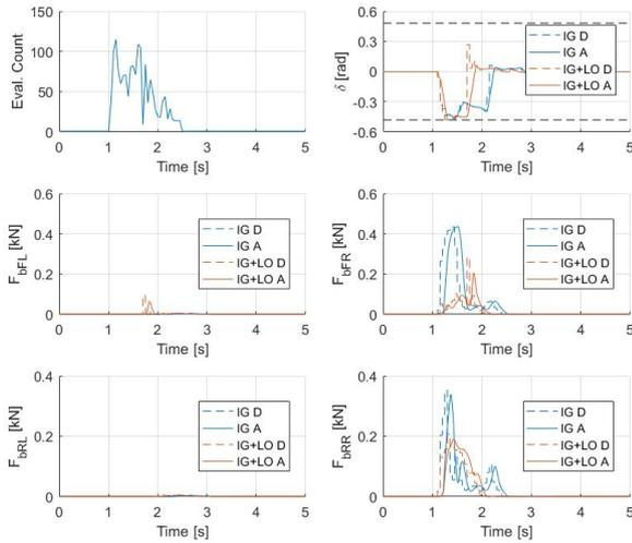
Fig. 10. Controller's action according to simulation with an initial speed of 126 km/h. The lateral impact was exerted at  $T=1.0s$ . NC for no control, IG for controlling with initial guess and IG+LO for controlling with NMPC. D for control demand and A for actual response of the actuators.
