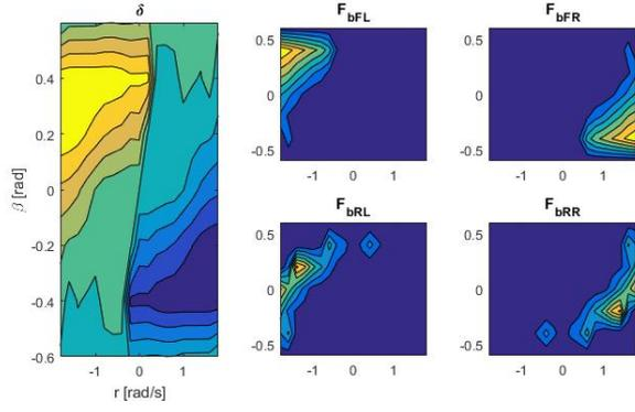
Fig. 4. The explicit control solution calculated with hybrid MPC. For steering, the yellow area means positive steering angle of the front wheels.
