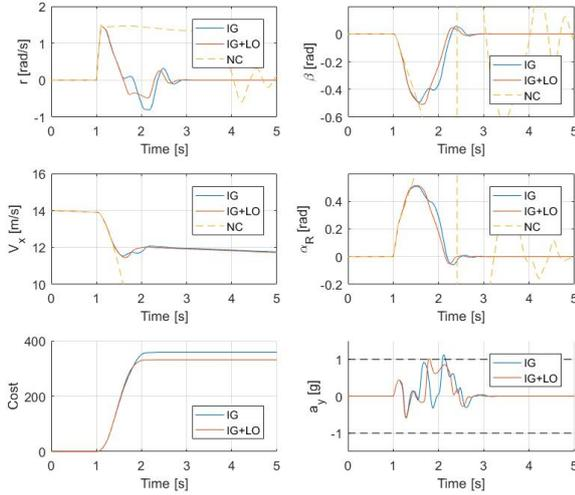
Fig. 7. Vehicle states according to simulation with an initial speed of 50 km/h. The lateral impact was exerted at  $T=1.0$ s. NC for no control, IG for controlling with initial guess and IG+LO for controlling with NMPC.
