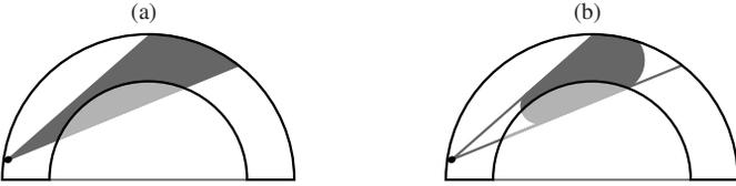
Fig. 2. The horizontal SVE for the baseline (a) and the augmented display (b). The baseline display shows two dimensional projections of constraints (called forbidden areas (FA)). The augmented display gives more precise constraints (called reduced forbidden areas (RFAs)) that take the dimension orthogonal to the projection into account. The differences on the VSD are similar to the differences on the HSD. The two display conditions are otherwise equal.
