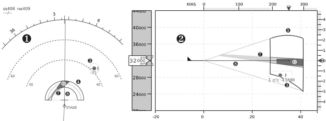
Fig. 1. Concept for a co-planar separation assistance display. This figure shows a HSD (①) and a VSD (②), with added separation assistance overlays. Relative intruder locations are indicated using TCAS-like symbology (③). ④ and ⑤ are the horizontal and vertical State-Vector Envelope, respectively. ⑥ is the reduced forbidden area on both on the HSD and the VSD. ⑦ is the projected forbidden area on both displays. ⑧ represents the ownship state vector.
