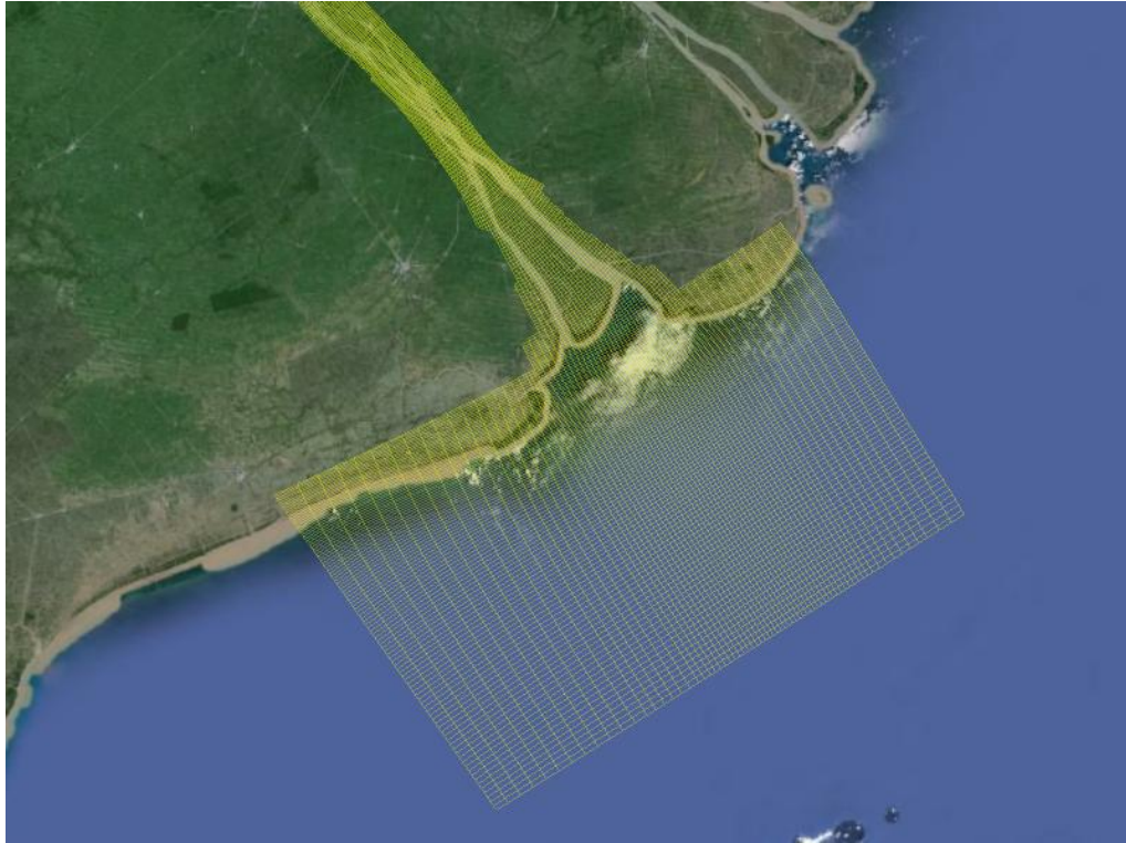
Figure 3.4: Grid of the model at the outer delta, river mouth and the most downstream part of the Hau river
