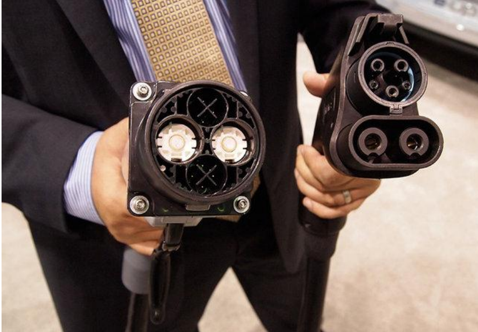
Figure 3.1: Two incompatible DC charging plugs: the CHAdeMO (left) and the SAE combined charger (right).
