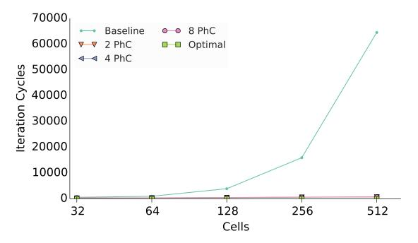
**Figure 5-8:** Comparison between different cluster sizes for different amounts of cells. The *normal* connection scheme is used and calculation times are *excluded* from the iteration times to show the pure network and administration costs. The systems use a router fan-out of two. The baseline is taken from [27].
