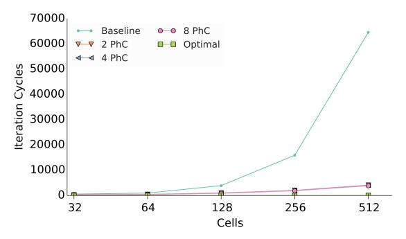
**Figure 5-7:** Comparison between different cluster sizes for different amounts of cells. The *complete* connection scheme is used and calculation times are *excluded* from the iteration times to show the pure network and administration costs. The systems use a router fan-out of two. The baseline is taken from [27].
