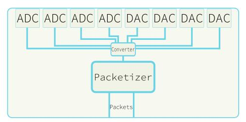
**Figure 3-8:** Diagram of the interface of the proposed system to the outside world. The system is used to enter analog data into the system and forward the data to specific cells. In return it receives data from the system and transmit the data back to analog signals.
