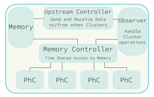
**Figure 4-1:** A cluster as used in the proposed system. The cluster allows for instant communication between any cells that are located inside the cluster. Each of the PhC time shares the calculation of multiple cells. The data of the cells that might be needed by other clusters is forwarded into a NoC.
