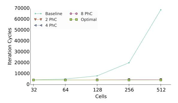
**Figure 5-11:** Comparison between different cluster sizes for different amounts of cells. The *normal* connection scheme is used and each cell calculation takes *534 cycles*. The systems use a router fan-out of two. The baseline is taken from [27]. All presented configurations of the new system meet the brain real time of 50 m at 100 MHz. Furthermore, all of them scale linearly with the number of cells. The Baseline on the other hand scales exponentially.
