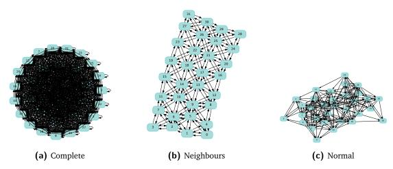
**Figure 5-6:** Examples of the different connection types used to test the iteration performance of the system. While the complete and neighbour calculations are static, the normal configuration is based on the normal distribution and cell distance and is newly generated for each simulation run. The results for the normal distribution are thus averaged over 10 runs to address for faster and slower configurations.
