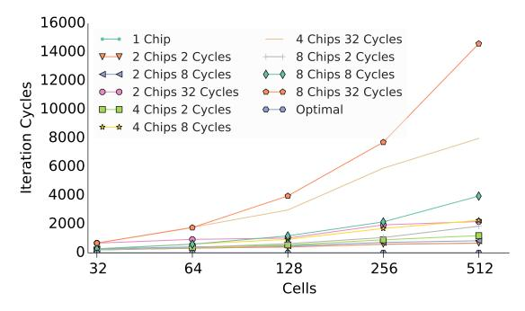
**Figure 5-13:** Comparison between different system configurations utilising between one and eight chips to simulate cell amounts between 32 and 512. Calculation times are *excluded*. The *normal* connection scheme is used. The multi chip systems utilise the packet based synchronization method.
