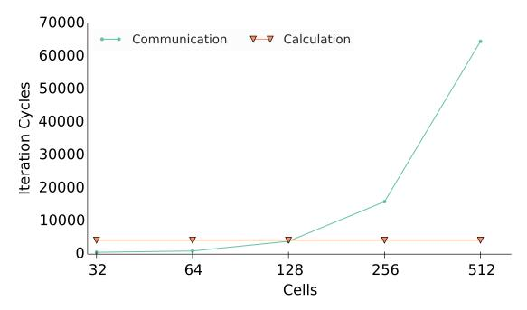
**Figure 1-1:** Time spent for the communication in each iteration of the extended Hodgkin-Huxley model in the implementation done in [27]. The system is limited by the communication cost which scales exponentially with the number of cells. To meet the brain real-time requirements, each iteration may only take up to 5000 cycles at 100 MHz clock speed.
