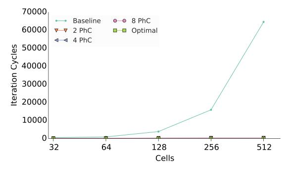
**Figure 5-9:** Comparison between different cluster sizes for different amounts of cells. The *neighbour* connection scheme is used and calculation times are *excluded* from the iteration times to show the pure network and administration costs. The systems use a router fan-out of two. The baseline is taken from [27].
