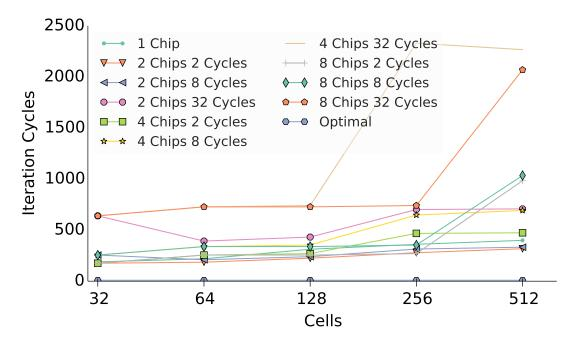
**Figure 5-18:** Comparison between different system configurations utilising between one and eight chips to simulate cell amounts between 32 and 512. Calculation times are *excluded*. The *neighbour* connection scheme is used. The multi chip systems utilise the dedicated wire based synchronization method.
