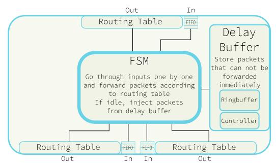
**Figure 4-2:** Diagram of a router as used by the proposed system. The routers are arranged in a tree topology. Each router has n children and except for the root router one upstream router. The router reads input packets from the input FIFO. Based on routing tables it determines where the packets have to be forwarded. If a receiving FIFO is full the packet is placed in the delayed buffer to be forwarded when the receiving router is free again.
