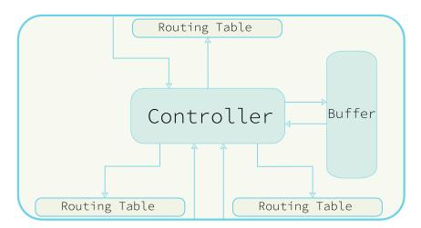
**Figure 3-6:** The abstract router described in Section 3-5. The controller queries each input and forwards packets according to the routing tables of the outputs. A packet may be forwarded into any direction and therefore each output has its own routing table. If a receiving router can not accept a packet that packet is stored inside the buffer till it can be forwarded.
