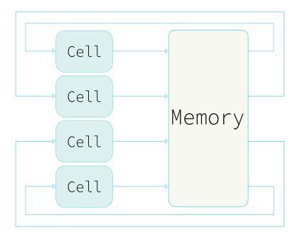
**Figure 3-2:** Optimal system with 4 cells utilising a shared memory. Each cell can write to and read from the shared memory. Thus, every cell is indirectly connected to any other cell. This system is not implementable in hardware as it requires too many memory ports and the wiring gets too complex.
