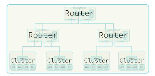
**Figure 3-5:** The complete network structure as designed in Sections 3-3 and 3-5. The computing elements PhC are grouped inside a cluster to make communication between neighbouring cells fast. These cluster are connected in a tree topology NoC. The router fan-out in this case is 2 and can be changed according to the requirements of the implementation. The same holds true for the number of PhC in any cluster.
