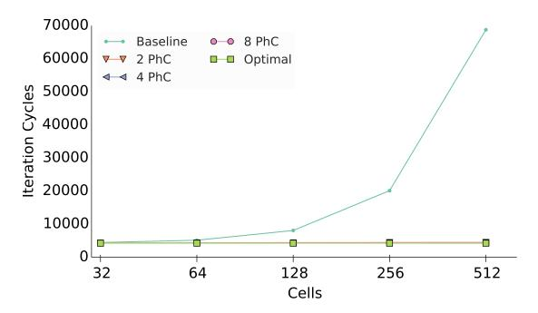
**Figure 5-12:** Comparison between different cluster sizes for different amounts of cells. The *neighbour* connection scheme is used and each cell calculation takes *534 cycles*. The systems use a router fan-out of two. The baseline is taken from [27]. All presented configurations of the new system meet the brain real time of 50 m at 100 MHz. Furthermore, all of them scale linearly with the number of cells. The Baseline on the other hand scales exponentially.
