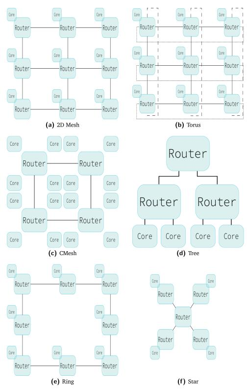
Figure 3-4: Typical topologies for a network on chip.
