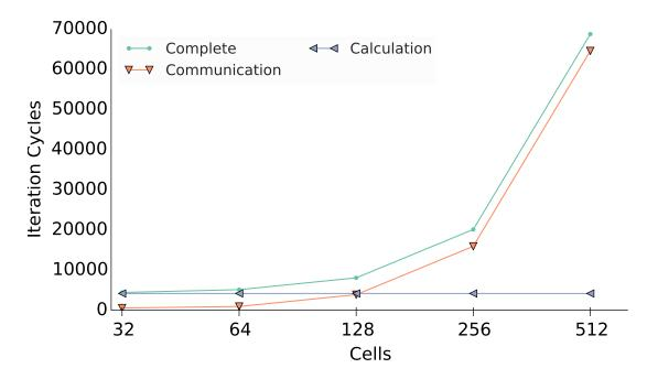
**Figure 2-1:** Amount of cycles required by the architecture to simulate the HH model as designed in [27]. As shown, the calculation time remains constant while the communication time scales exponentially with the amount of cells in the system.
