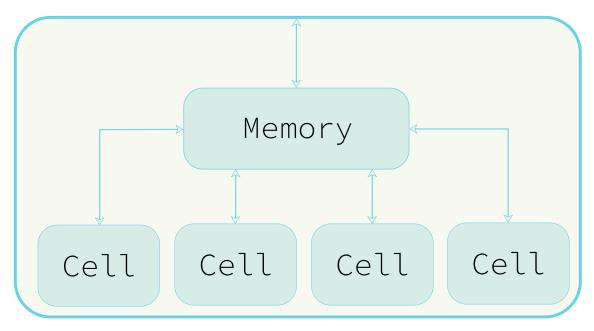
**Figure 3-3:** Abstract design of a cluster. PhC are grouped around a central shared memory. The cluster is connected to other clusters using an interconnect.
