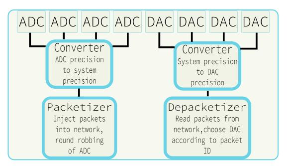
**Figure 4-3:** Part of the system that interfaces with the outside world. The date from the converters is put into packets and routed down the tree to the correct clusters. In return clusters can send packets up the stream to the output converters.
