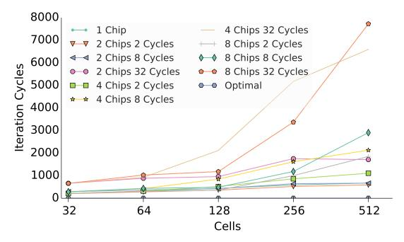
**Figure 5-17:** Comparison between different system configurations utilising between one and eight chips to simulate cell amounts between 32 and 512. Calculation times are *excluded*. The *normal* connection scheme is used. The multi chip systems utilise the dedicated wire based synchronization method.
