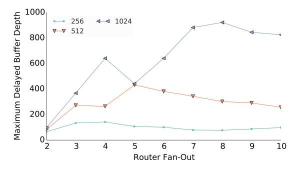
**Figure 5-2:** Comparison of maximum delayed packet buffer depths for different router configurations. This graph shows that the delayed buffer strategy is feasible without large delayed buffers for lower router fan-outs. Clusters are kept at two PhC with 8 shared cells. The number of cells and thus clusters and routers in the system is varied between 256, 512 and 1024.
