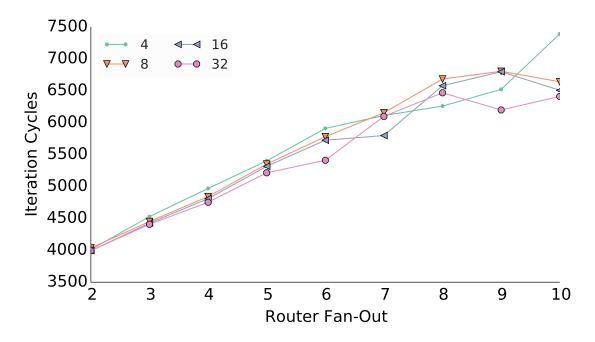
**Figure 5-1:** Comparison of the system's iteration performance for router input FIFO depths of 4,8,16 and 32 elements. All clusters have 2 PhC and the router fan-out are varied between 2 and 10.
