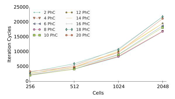
**Figure 5-5:** Comparison of systems with different cluster sizes. The routers are kept constant at a fan-out of two. Clusters with two, four and eight PhC achieve the best iteration times while larger clusters are generally slower especially at 512 cells.
