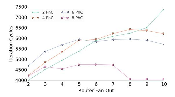
**Figure 5-4:** Comparison of iteration performance for 512 cells and different cluster sizes. Except for large clusters with eight cells small routers perform better than large routers. The overall best performing configuration consists of small clusters and small routers at two PhC per cluster and a fan-out of two.
