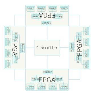
**Figure 3-7:** This figure shows the multi-FPGA system described in Section 5-3. The single FPGA (Sections 3-3 and 3-5) implementations are connected using a ring topology network. The FPGA are synchronized via a central controller with two wires. One of the wires indicates when the corresponding FPGA is done and the other wire is used by the controller to indicate a new iteration.
