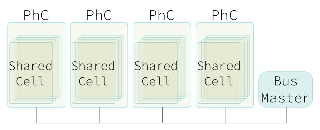
**Figure 2-2:** HH simulator as designed in [27]. The Physical Cells (PhCs) simulate multiple neurons in a time shared fashion. They are connected by a shared bus, which is controlled by the bus master.
