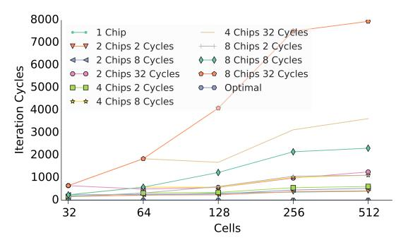
**Figure 5-14:** Comparison between different system configurations utilising between one and eight chips to simulate cell amounts between 32 and 512. Calculation times are *excluded*. The *neighbour* connection scheme is used. The multi chip systems utilise the packet based synchronization method.
