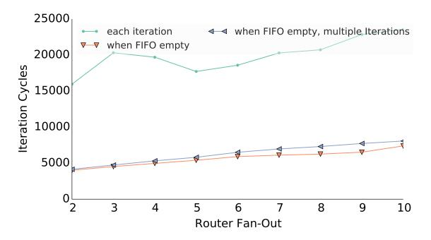
**Figure 5-3:** Comparison between three delayed packet injection schemes. Injecting the packets after each round through all input FIFO results in the slowest iteration times. Injecting only when all FIFO are empty for one round or for multiple rounds achieves comparable performance but injecting after one round of input inactivity results in the best overall performance.
