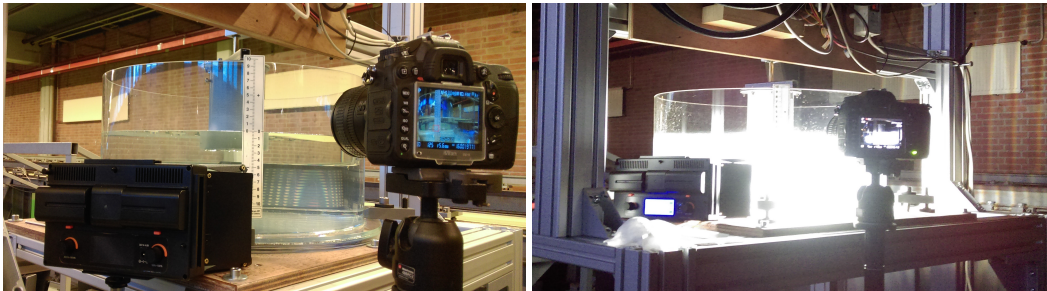
FIGURE 6.25: Video camera placed next to water container and the achieved contrast between water and ambient air
