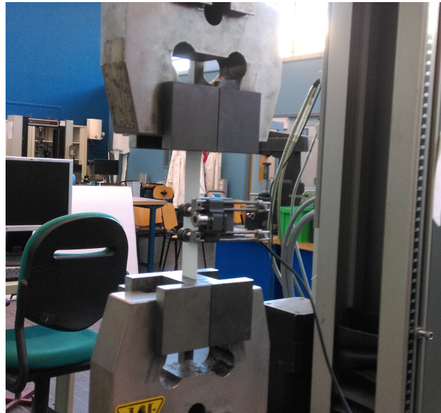
FIGURE B.1: PTFE specimen clamped with a digital extensometer attached
