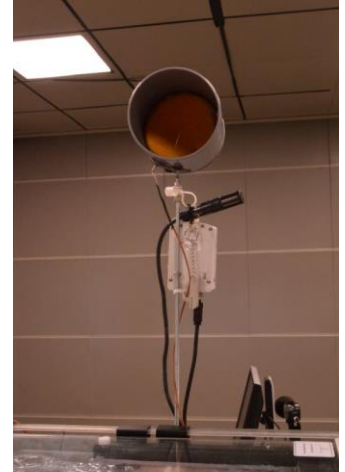
Fig. 12. Configuration of the thermocouple and humidity sensor.
