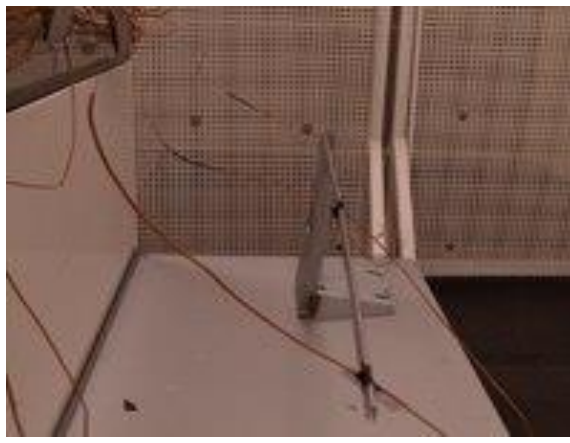
Fig. 25. Thermocouple frame that measures the spilled air temperature.
