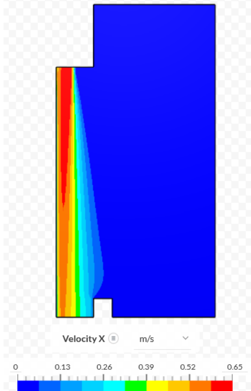
Fig. 51. Contour plot of the velocity in the x direction for the isothermal air curtain.
