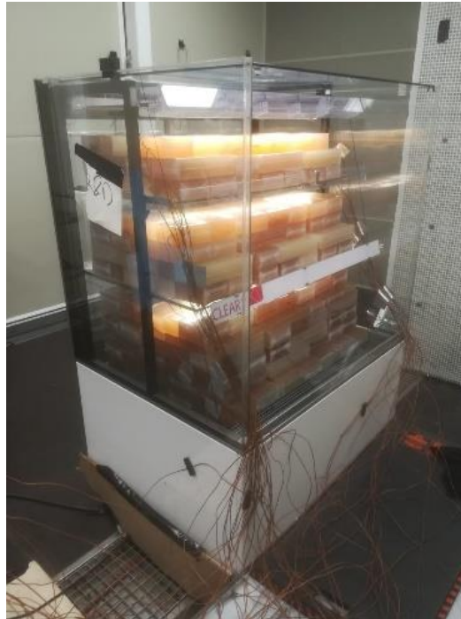
Fig. 1. The studied cabinet: MCC COLD 90 ss in the climate chamber, during the experimental testing.
