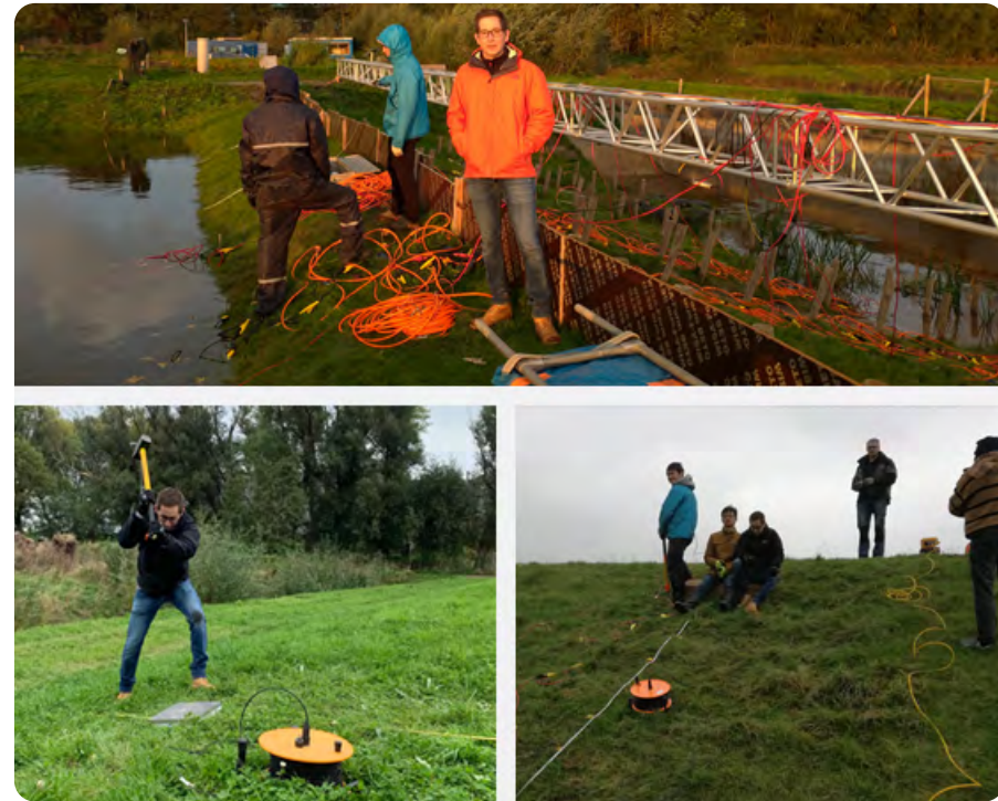
Figure 2: Geophysical survey in dikes and associated instrumentation. Photos by Juan Chavez Olalla.
