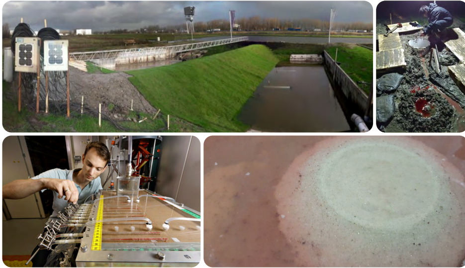
Experiments on pipe development. Top left: large-scale test in the Flood Proof Holland facility at the TU Delft. Top right: measurements during the large-scale test. Bottom right: sand boil in the large-scale test. Bottom left: small-scale experiments. Photo © Sam Rentmeester.
