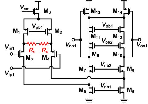
Fig. 11. Source degenerated OTA of the 2nd integrator.
