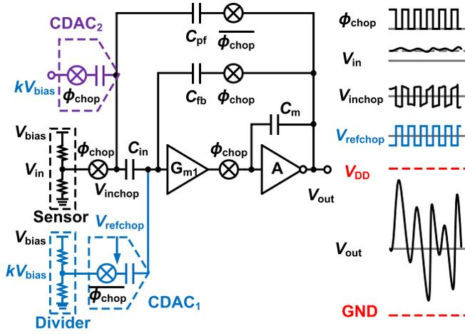
Fig. 4. Block diagram of the CCIA illustrating the operation of the bridge offset compensation and dual-path input impedance boosting loops.
