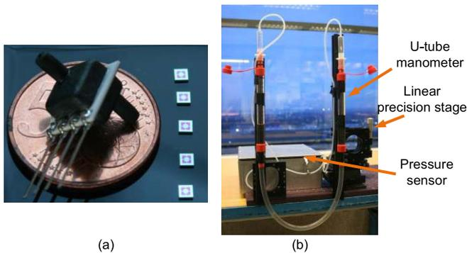
Fig. 16. (a) AC4010. (b) Differential pressure measurement setup.
