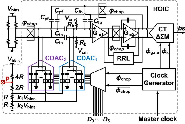
Fig. 6. Simplified circuit diagram of the bridge ROIC.
