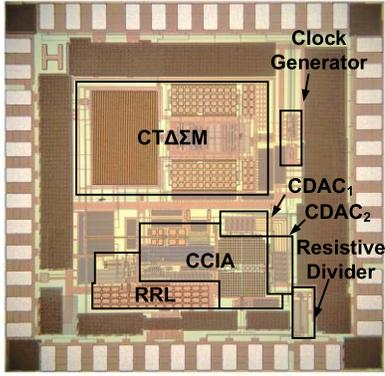
Fig. 12. Micrographs of the ROIC.
