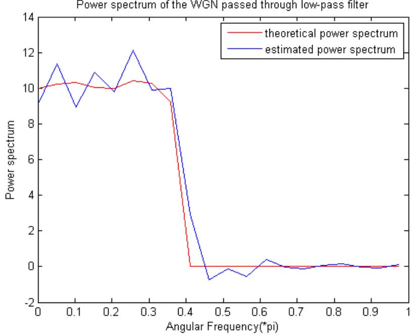
Figure 6.7: Power spectrum of the WGN passed through low-pass filter
