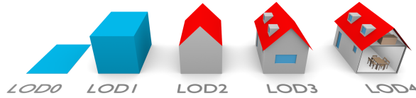
Figure 6.3: A building represented in LOD0 to LOD4 in CityGML (Source: Biljecki et al. [18])
