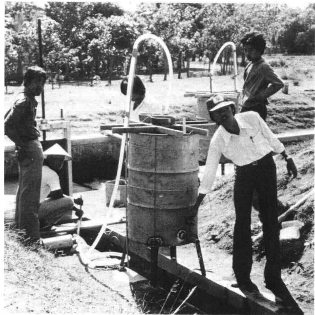
Figure 3 Monitoring field performance of vortex tube in Java
