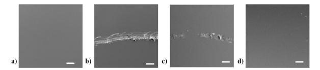
Figure 2: Self-healing experiment of copolymer **P7**. a) Film after crosslinking, b) scratch before annealing, c) scratch after annealing at 160 °C for 1 min and d) scratch after annealing at 160 °C for 3 min (scale bars = 100  $\mu$ m).
