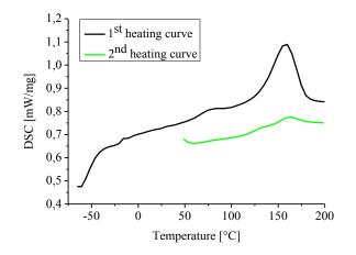
Figure 1: DSC analysis of copolymer **P7**.
