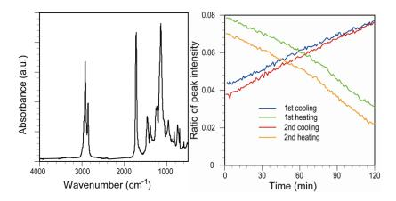
Figure 3: (a) FTIR spectra of the crosslinked polymer prior to the heating and cooling cycles. For quantitative analysis, the peak height ratio of the furan ring breathing at 1065 cm<sup>-1</sup> to the carbonyl stretch at 1724 cm<sup>-1</sup> was calculated, and (b) cycling between temperatures of 40 and 160 °C show reversible appearance and disappearance of the furan peak. For each cycle, the temperature was held constant for 120 min.
