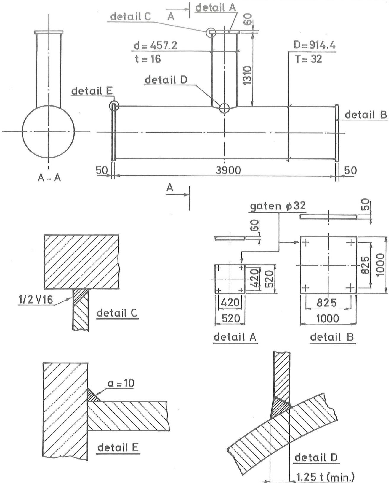
Figuur: 4 Tubular T-joint specimen
