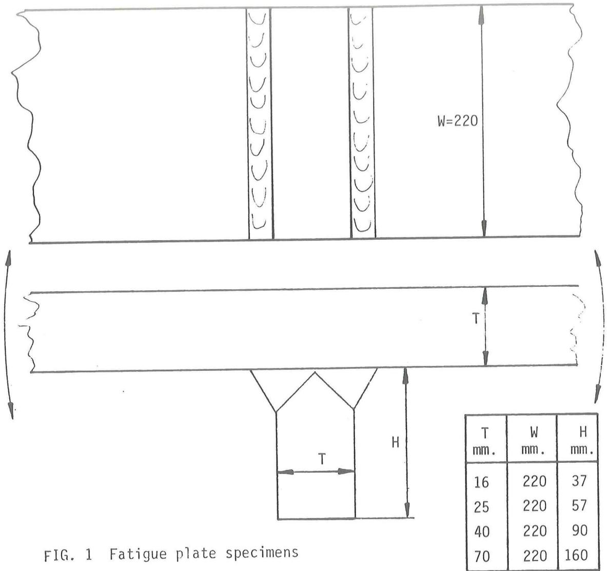
FIG. 1 Fatigue plate specimens
