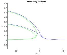
Figure 5.3: Hardening cubic Duffing oscillator.
