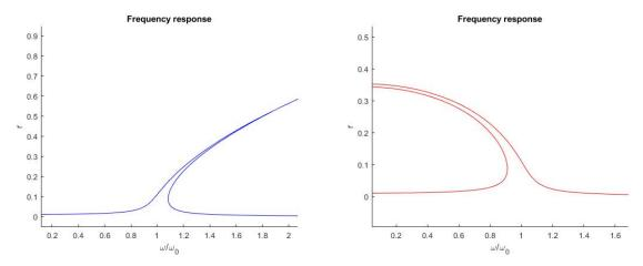
Figure 5.10: Hardening system,  $\alpha, \psi > 0$ .
