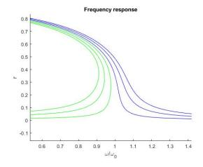
Figure 5.5: Hardening quintic Duffing oscillator, vaying damping coefficient.
