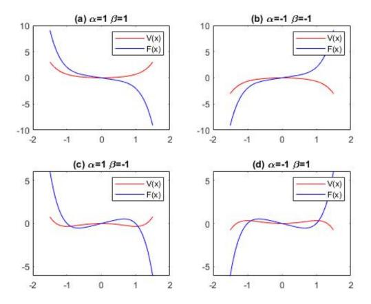
Figure 3.1: Potential and force of the undamped system for different values of  $\alpha$  and  $\beta$
