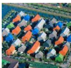
U14. Ypenburg masterplan MVRDV , The Hague, NL Island Area: 2.0 ha FSI = 1,07 GSI = 0,39 OSR = 0,56 L = 2,72
