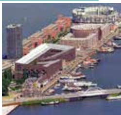
U5. KNSM Island, Amsterdam, NL Island Area: 3,3ha FSI = 4,17 GSI = 0,64 OSR = 0,09 L = 6,50
