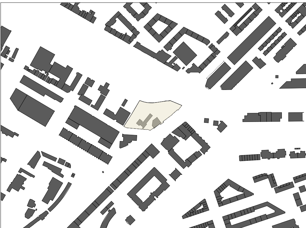
Figure 31 - Figure Ground drawing - This map indicated built and unbuilt areas in the location. The location itself is marked with a brownish colour with black dotted lines. It is clear to see that there is no clear structure in the area and that the buildings all are like single entities. The location therefore allows with a lot of options to design various building masses - Source: Own Image
