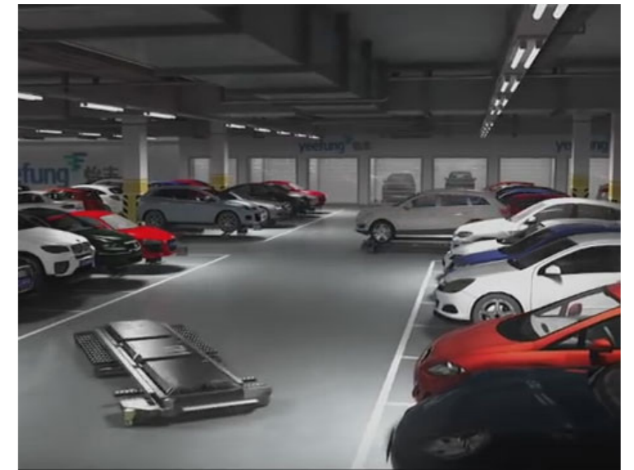
Robotized trolley collecting a car. The Robot can rotate on his axis so the turning radius is therefore the same as the length of the trolley itself. Source: https://bit.ly/29pMC4b
