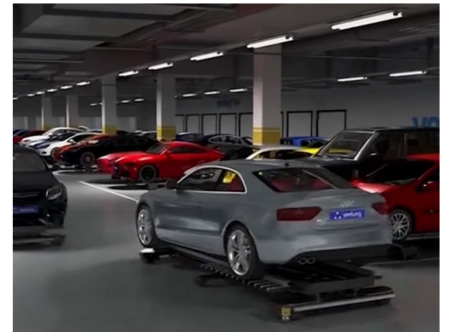
The cars are all parked on simple platforms and stored away. The robot fits perfectly underneath and lift the platform up slight to maneuver it. Source: https://bit.ly/29pMC4b
