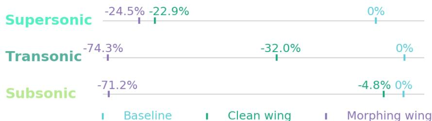
Figure 5.8: Comparison between clean and morphing wing drag improvement at different flight conditions for the test cases reported in Fig. 5.6 and Fig. 5.7.
