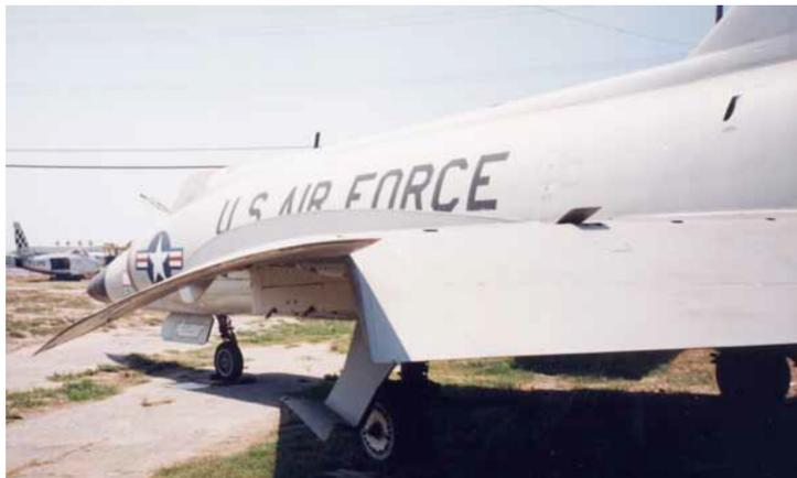
Figure 1.4: Detail of F-102 wing showing the conical camber of the leading edge, by Prof. Mason [41]. According to the author, this feature is so evident because it was added at a later design stage, with a trial-and-error approach typical of these early supersonic aircraft projects.
