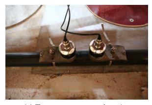
(a) Two sensors connected to pipe
