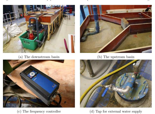
Figure A.1: Sections at the upstream side of the flume.
