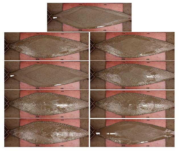
Figure B.4: Photo's taken at distinctive moments during the experiment. Starting up top: formation island.
