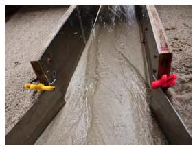
Figure 3.7: The overlap and connection between the different sections causes some local perturbations.
