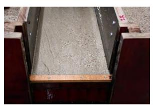
(a) Upstream installed weir
