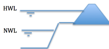
Figure 158: Cross - section dike principal
