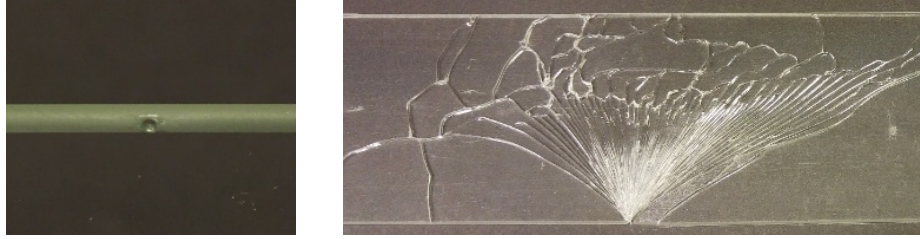
Fig. 4 Detail of a flaw on the edge of the sample tested and corresponding cracking pattern
