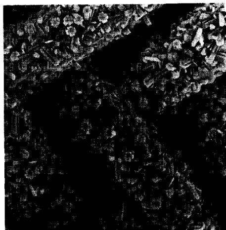
Figure 1-5 MFI crystals, in situ grown on metal wire gauze with a wire diameter of 35 \mu\text{m} and a mesh size of 40 \mu\text{m} .
