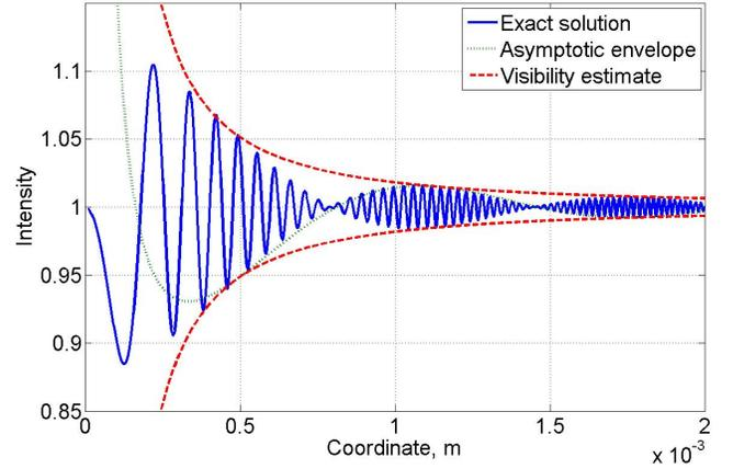
**Fig. 2.** Fringe intensity calculated for  $r = 25 \mu\text{m}$ ,  $L = 0.05 \text{ m}$  and  $\lambda = 0.65 \mu\text{m}$  according to the exact formula Eq. 3, and using the asymptotic approximations 4 and 5.
