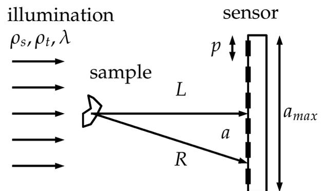
**Fig. 1.** Schematic of a holographic microscope. The sample is illuminated with a plane wave with wavelength  $\lambda$ , having spatial coherence size of  $\rho_s$  and the temporal coherence length of  $\rho_t$ . The diffraction pattern is registered by a sensor with pitch  $p$  at a distance  $L$ .
