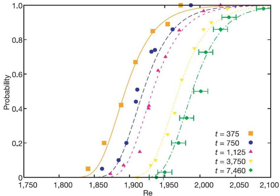
Figure 2.11: Probability distribution obtained by Hof et al. (2006) showing clearly the S-shaped curves
