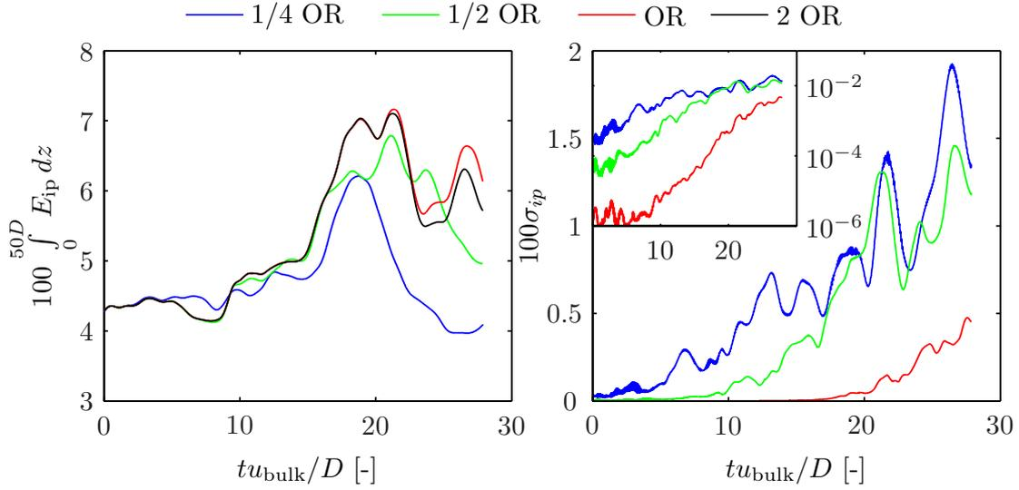
Figure 5.3: *left* Development of the total in-plane kinetic energy over time. *right* Standard deviation of the in-plane kinetic energy with respect to the 2 OR case. *inset* Standard deviation on a logarithmic scale.
