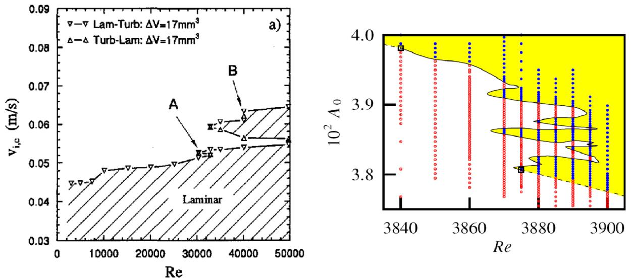
Figure 1.3: *left* experimental results by Draad (1996) on the critical amplitude to trigger turbulence. The shaded area indicated the return to laminar flow *right* similar result for numerical simulation by Schneider, Eckhardt and Yorke (2007). Be aware that here the shaded area indicates a transition to turbulence
