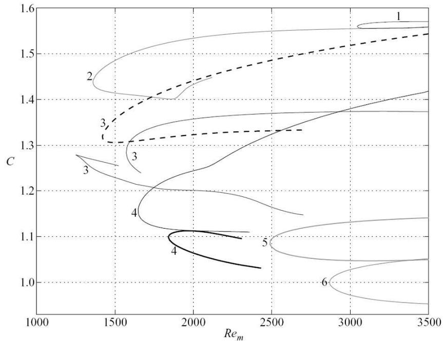
Figure 2.2: The phase speed of traveling waves (the number indicates the rotational symmetry) relative to the mean bulk velocity as a function of the Reynolds number. From: Wedin and Kerswell (2004).
