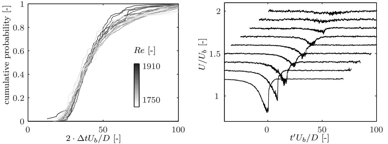
Figure 4.6: *Left* Cumulative probability distribution of the time needed between initiation and complete decay of a puff; *Right* Evolution of the conditionally-averaged centerline velocity of a decaying puff for nine consecutive times relative to the onset of decay ( $t_5$  in figure 4.2).
