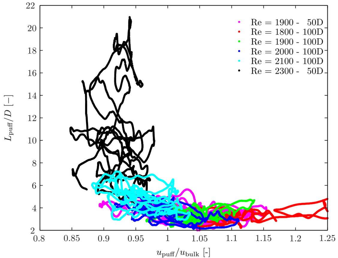
Figure 5.11: The correlation between the length of the puff and its instantaneous velocity. The length of the puff does not depend on the velocity of the puff. For  $Re < 2100$  the velocity is bounded to  $\approx 5D$ . This boundary is breached when  $Re > 2000$ . Only the data for  $Re = 2300$  for time  $tu_{\text{bulk}}/D < 500$  are taken into account, this is just before this structure splits into two puffs.
