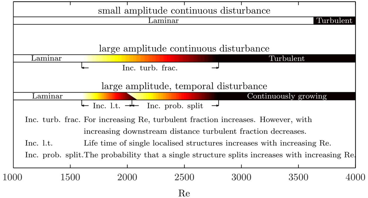
Figure 1.4: Depending on the type of disturbance, different flow patterns emerge downstream of the disturbance
