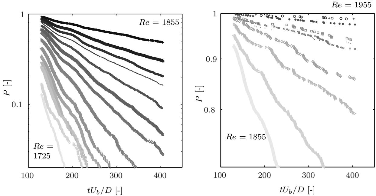
Figure 4.4: Semi-log plots of the probability  $P(t; Re)$  that a puff survives a time  $t U_b/D$ , where  $U_b$  is the bulk velocity and  $D$  the pipe diameter, for  $Re$  between  $1725 \pm 5$  and  $1955 \pm 5$ , in increments of 10. The data for  $Re=1855$  appears in both graphs for reference. The slope of each curve determines  $\tau(Re)$  defined in (4.1), which increases with  $Re$ .
