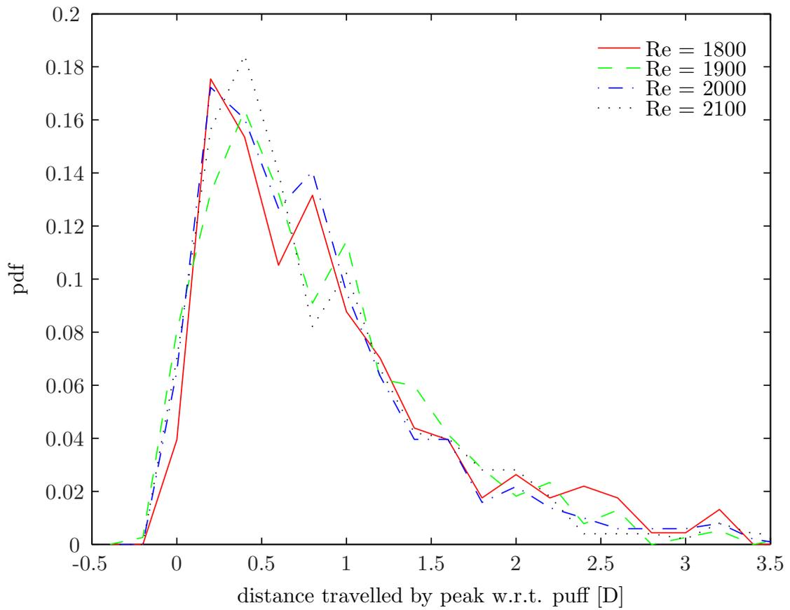
Figure 5.15: The distance covered by the peaks with respect to the puff. The distance that is travelled with respect to the puff seems to be independent of the Reynolds number.
