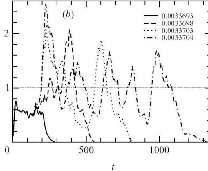
Figure 2.4: Time series of the disturbance energy for four slightly different initial conditions for a pipe flow at  $Re = 2,000$ , showing the large variation of life time. From: Faisst and Eckhardt (2004)
