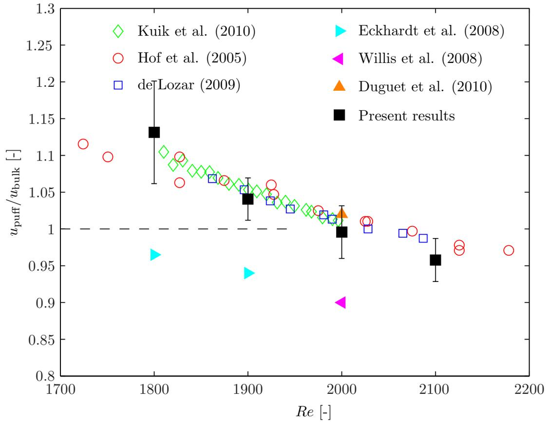
Figure 5.9: Average velocity of a puff as a function of the Reynolds number. Results obtained by experiments are given by open symbols, while filled symbols are the results from numerical simulations. The error-bars indicate the actual variation in puff velocity and is determined by taking the standard deviation of the mean instantaneous puff velocity.
