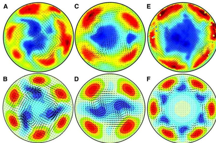
Figure 2.1: Comparison of experimental data of instationary pipe flow in a planar cross section (A-C-E) and corresponding exact traveling wave states (B-D-F). From: Hof et al. (2004).
