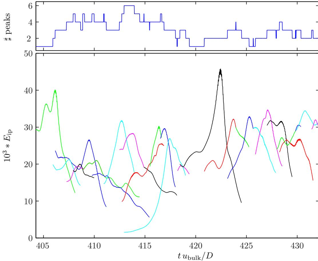
Figure 5.12: The development of the amplitude of a peak over time. Only the peaks that once become the global maximum are taken into account *Top* the number of identified peaks that are simultaneously present over time.
