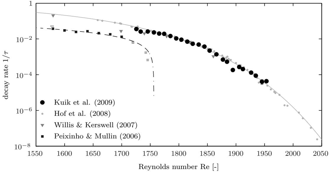
Figure 2.12: The life time of decay rate for  $P(t)$  as a function of Reynolds number. After: Kuik et al. (2010)
