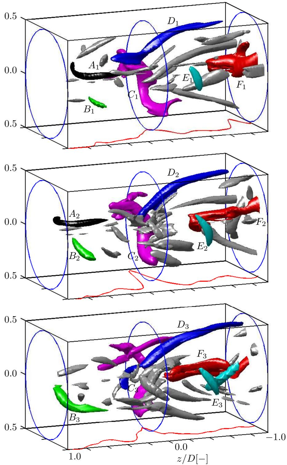
Figure 5.16: Coherent structures in a puff in a convective reference frame that moves along with a peak. The time between consecutive images is  $t u_{\text{bulk}}/D = 0.7$  timescales. Coherent structures are visualized using iso-contours of  $Q$ . On the bottom of each figure the in-plane kinetic energy distribution is shown as a reference.
