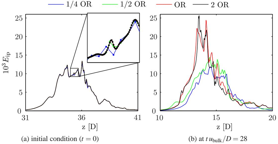
Figure 5.2: Distribution of in-plane kinetic energy: (*left*) initial condition, (*inset*) a part of the curve is enlarged to highlight differences in the initial condition; (*right*) after continuation over  $t u_{\text{bulk}}/D = 28$ , for four different spatial resolutions. Flow is from left to right. The values indicating the axial location shows smaller values in the right part, because of passing the periodic boundary.
