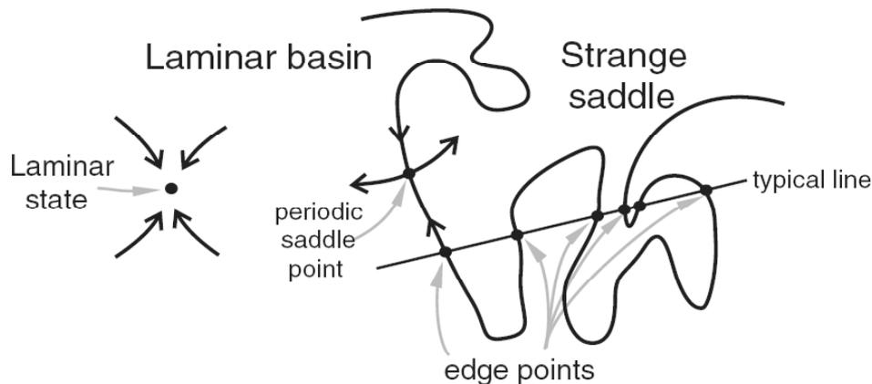
Figure 2.3: Schematic representation of phase space in pipe flow. The laminar flow state is an attractor by increasing the Reynolds number its basin of attraction reduces, if the flow is perturbed outside the basin of attraction, the flow wanders around the traveling wave solutions found by Wedin and Kerswell (2004), Faisst and Eckhardt (2003). Courtesy of: T. Schneider, Univ. Marburg.
