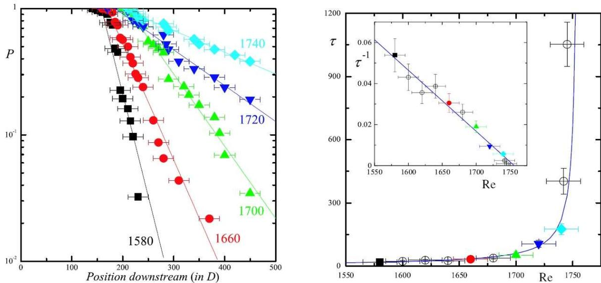
Figure 2.6: (left) Probability of observation of a puff versus downstream distance. (right) Mean decay rate as a function of  $Re$ . The inset shows the inverse life time with a linear fit indicating  $Re_c \approx 1750 \pm 10$ . From: Peixinho and Mullin (2006)
