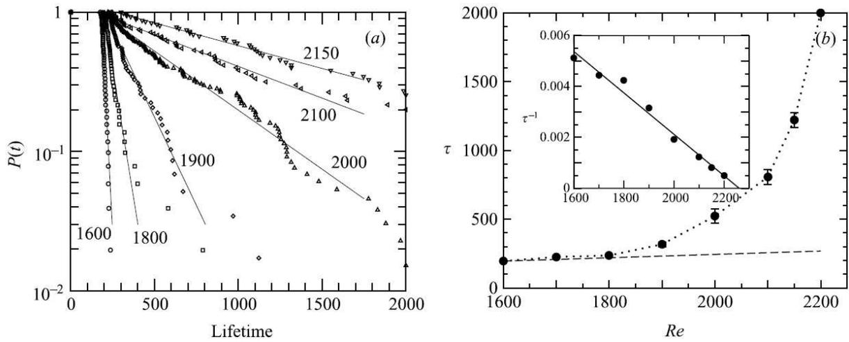
Figure 2.5: Turbulent life times as a function of Reynolds number. (left) Probability  $P(t)$  for a single trajectory to still be turbulent after a time  $t$ . (right) Median  $\tau$  of the turbulent lifetimes as a function of Reynolds number. The inset shows the reciprocal median lifetime vs.  $Re$  and a linear fit, corresponding to  $\tau(Re) \propto (Re_c - Re)^{-1}$ , with  $Re_c \approx 2250$ . From: Faisst and Eckhardt (2004)
