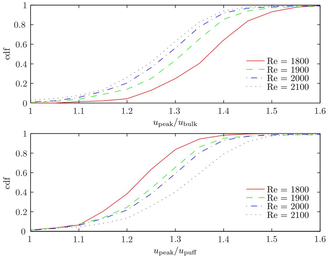
Figure 5.14: Cumulative distribution of the velocity of a peak for different Reynolds numbers, relative to the bulk velocity (*Top*) and to the puff velocity (*Bottom*). The peaks move slower with respect to the bulk velocity for increasing Reynolds number. The opposite behavior is observed with respect to the puff velocity.
