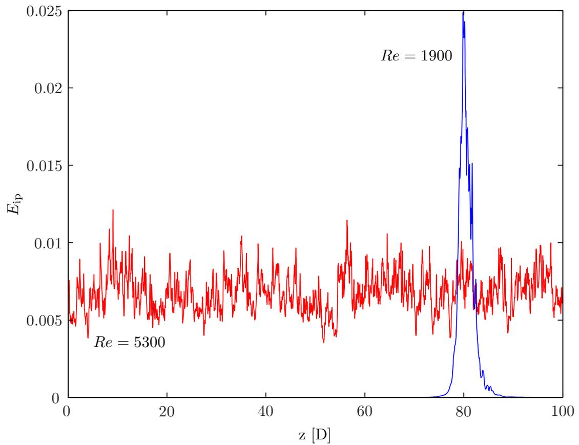
Figure 5.6: The kinetic energy of the in-plane velocity components for fully developed turbulent pipe flow ( $Re = 5300$ ) and localized turbulence occurring the form of a puff ( $Re = 1900$ )
