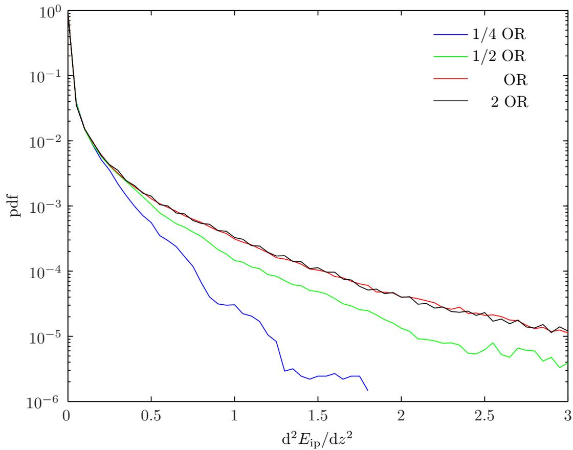
Figure 5.4: Probability distribution of the second derivative of the in-plane kinetic energy distribution for four different resolutions. This shows clearly that the simulations at the lower resolutions (i.e. 1/2 OR and 1/4 OR) are not able to resolve all small scale features of the distribution.
