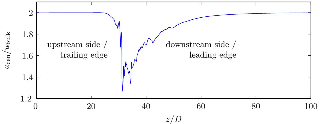
Figure 1.5: Centerline velocity in a domain with a single puff present. The flow is in positive  $z$  direction. In the figure the definition for the leading and trailing edge of the puff are given.
