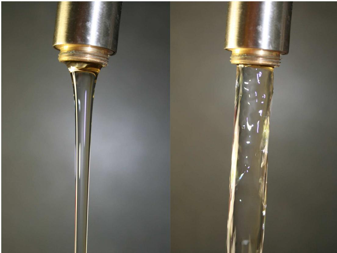
Figure 1.1: The flow of water from a tap in our kitchen: In the left part the flow shows a nice undeformed state. Here the fluid elements are all moving in parallel and this state is known as the laminar state. As the flow rate is increased, the flow becomes turbulent and irregular, random motion is observed.
