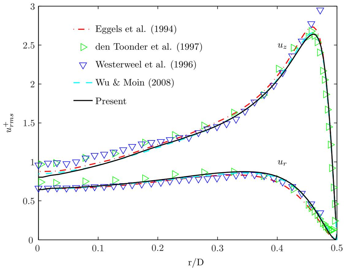
Figure 5.5: Profiles for the axial ( $u_z$ ) and radial ( $u_r$ ) velocity fluctuations as simulated by Eggels et al. (1994) and Wu and Moin (2008), measured by Westerweel et al. (1996) and denToonder and Nieuwstadt (1997) and the present simulations.
