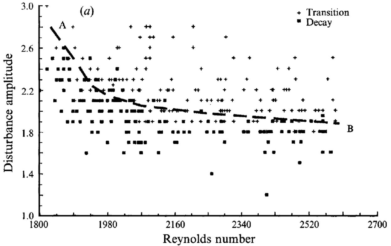
Figure 1.2: The results of the experiments by Darbyshire and Mullin (1995) to determine the critical amplitude required to trigger turbulent flow.
