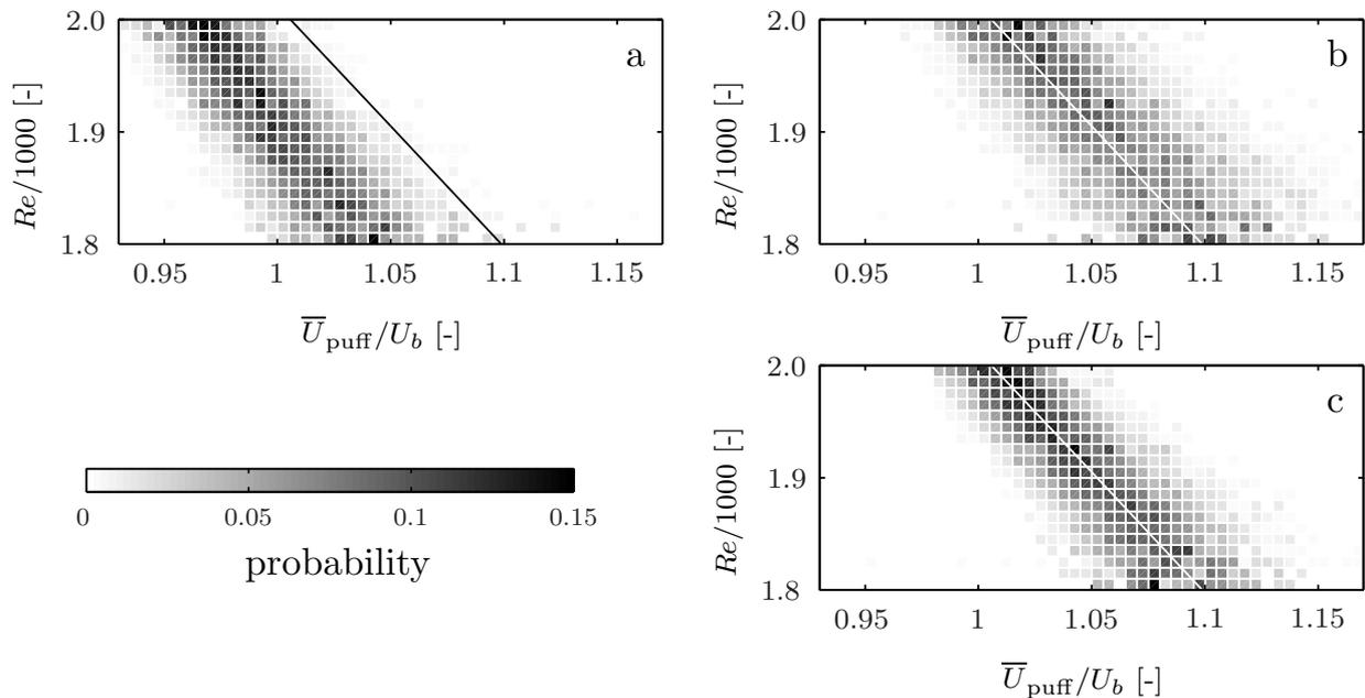
Figure 4.3: Probability density functions of relative average puff velocity as a function of  $Re$ ; (a) in section  $S_1$ ; (b) in section  $S_2$ ; (c) in section  $S_3$ . The inclined straight line is a least square fit to the velocity distribution in section  $S_2$  and is given in the other plots for comparison.
