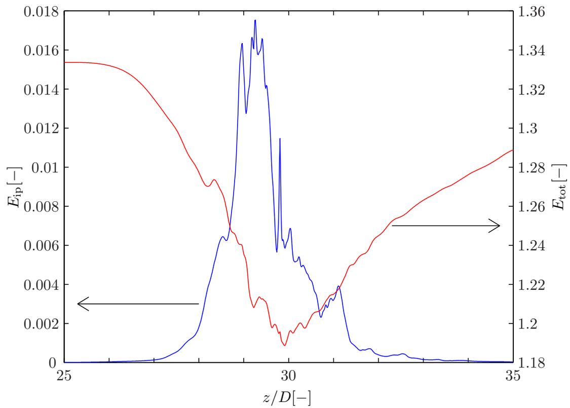
Figure 5.1: Distribution of the total kinetic energy  $E_{tot}$ , as defined in (5.3) and the contribution to the kinetic energy by the in-plane velocity components only  $E_{ip}$  (5.4)
