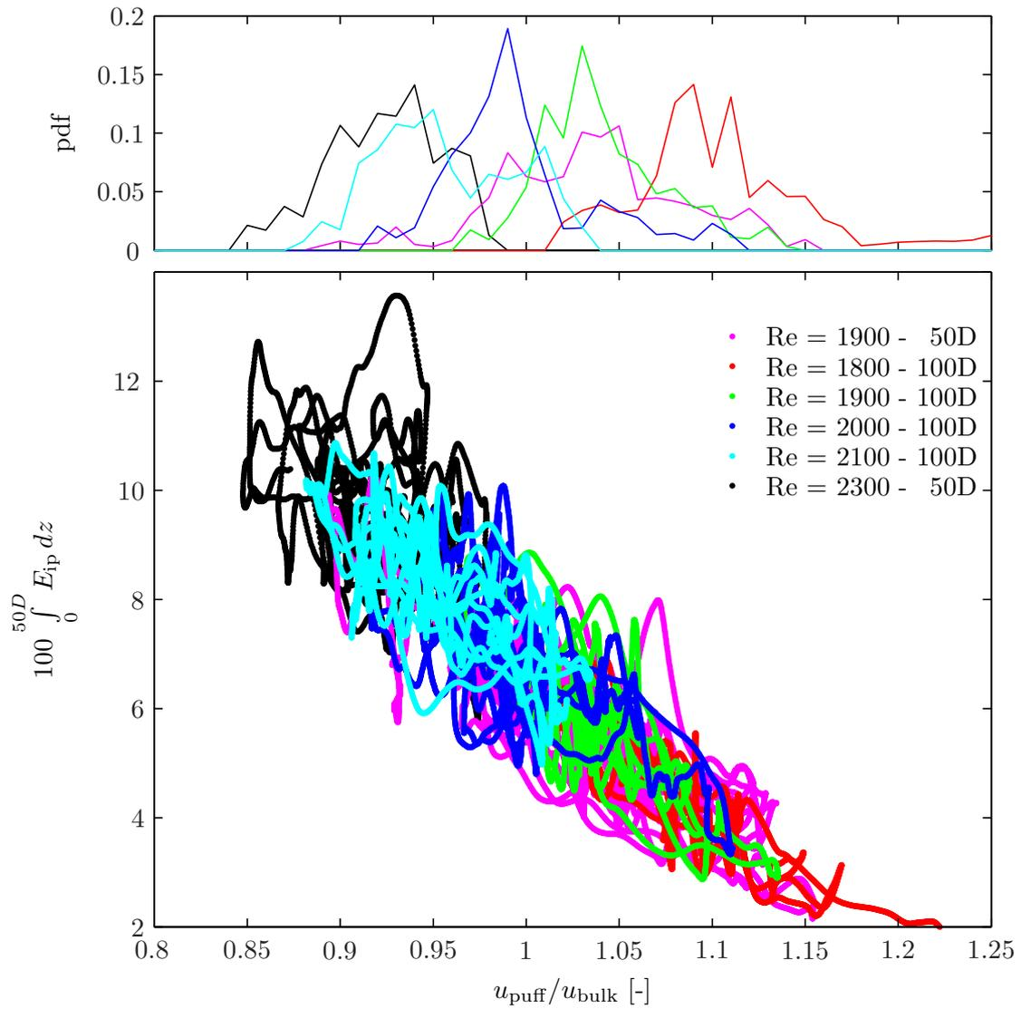
Figure 5.10: The correlation between the instantaneous velocity of a puff and the total in-plane kinetic energy. Only the data for  $Re = 2300$  before the structure splits into two separate puffs are considered in this figure. It seems that the behavior of the puff is independent of Reynolds number and that the velocity is determined by the total amount of in-plane kinetic energy.
