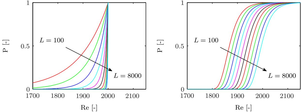
Figure 2.10: *left* probability as a function of Reynolds number if  $\tau^{-1} \sim (Re_c - Re)$ , with  $Re_c = 2000$  *right* probability as function of Reynolds number if  $\tau^{-1} \sim \exp(Re)$
