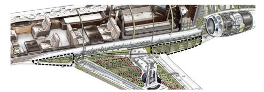
Figure 1.9: Cutaway of Dassault Falcon 8X showing fuel tanks in the wing-body fairing [33]
