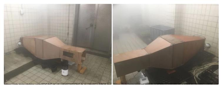
With all the section built, made water resistant, screws for the springs, and airstrips in place it is time for to assemble them all.
