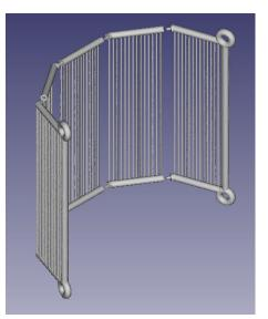
3D model of curved fog catcher prototype. The five seperate parts can be put together with a pins on some parts and holes in others. DEPENDING ON HOW THEY WERE FACING THE FOG STREAM.
