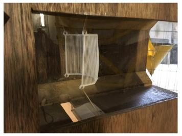
Curved prototype suspended inside the test section of the wind tunnel. At the bottom of the wind tunnel a 3D printed slanted plate is plate to ensure drainage of all water droplets shedding of the net.
