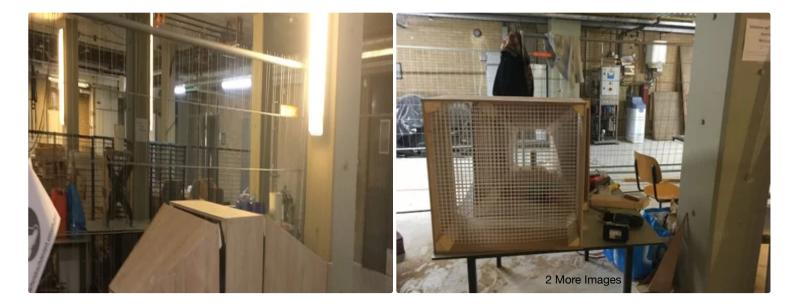
These three sections are the most straightforward to build, so a good place to start. All three follow a similar process, the only difference is that you need to add the egg crates to the straightener section.
