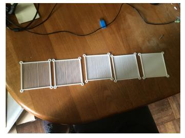
First five straight fog catcher prototypes with varying shade coefficients.
