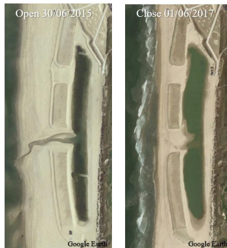
Figure 3-9: Satellite imagery from Google Earth. Left image shows an open channel, right shows a closed channel.
