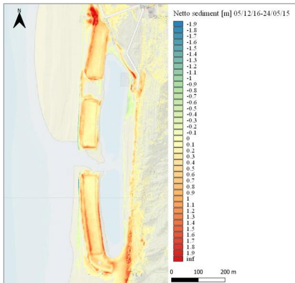
Figure 0-4: Sediment change lagoon area above 2 m NAP, between 05/12/16-24/05/15. Blue corresponds to erosion, red corresponds to accreting, yellow shows no changes.
