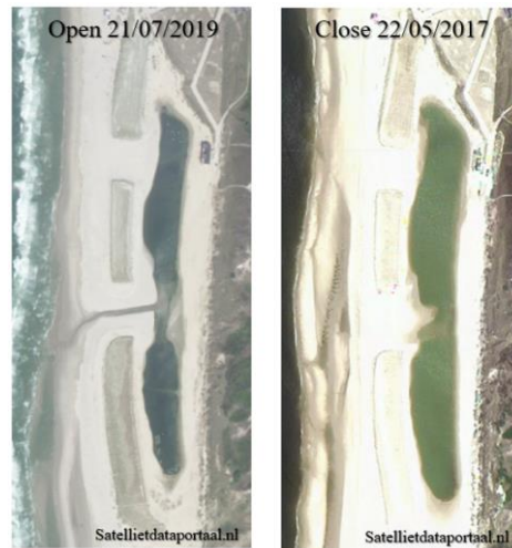
Figure 3-11: Satellite imagery from Satellietdataportaal.nl. Left image shows an open channel, right image shows a closed channel.
