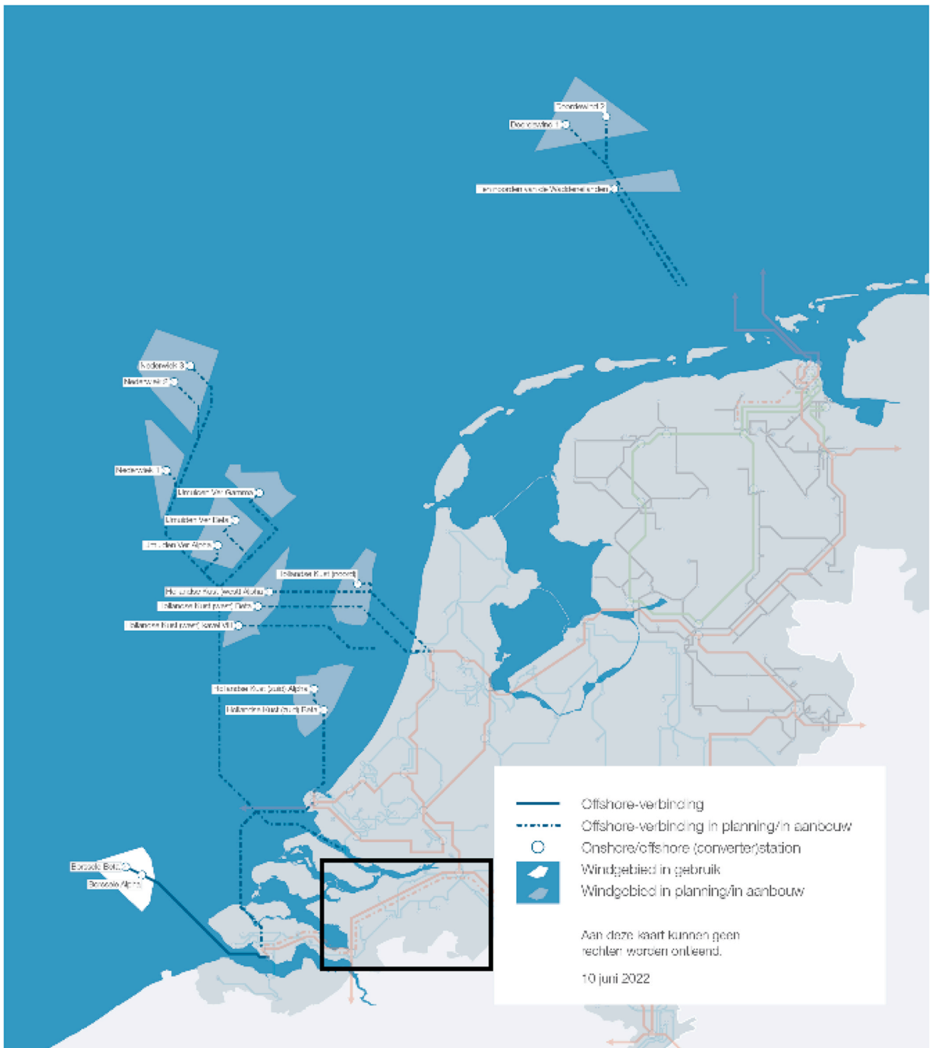
Fig. 1. Location of the transmission route connecting the offshore wind farms, through the province of Zeeland towards the city of Tilburg. Source: https://www.tennet.eu/nl/projecten/offshore-projecten-nederland , accessed 19-01-2023.
