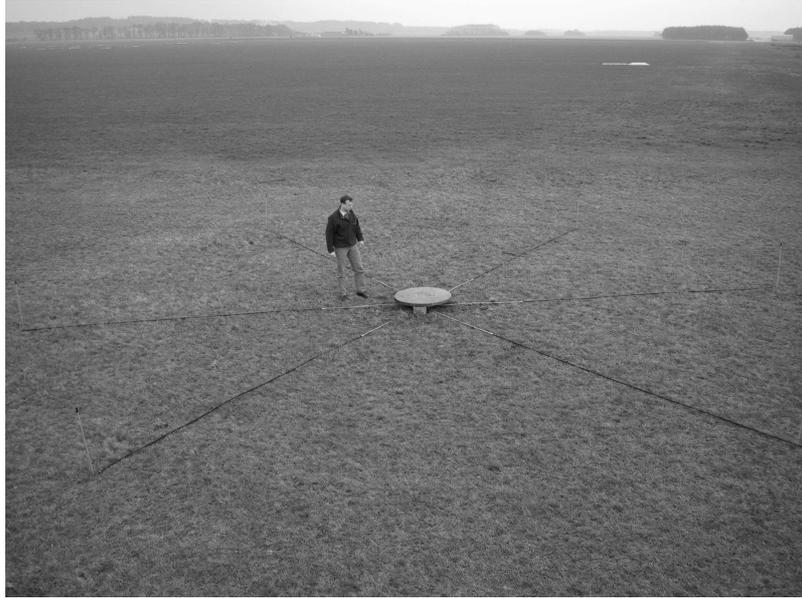
**Figure 2.6:** Installation of a microbarometer in DIA. The microbarometer is installed beneath the earth's surface and covered by a concrete top. The atmosphere is sampled by six porous hoses in a star-like layout, each of 5 m length.
