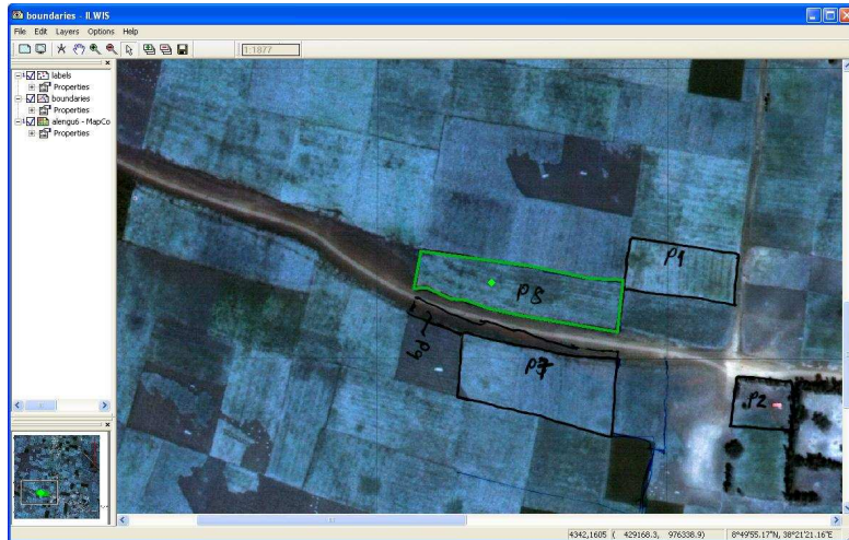
Figure 14: Presentation of parcels - shown in green lines in ILWIS /Postgres based STDM
