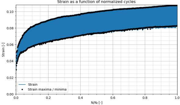
Strain as a function of normalized cycles
