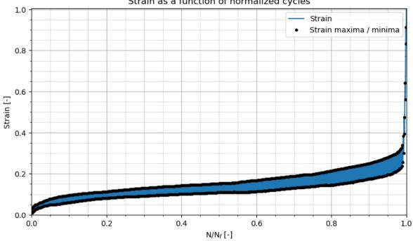
Strain as a function of normalized cycles
