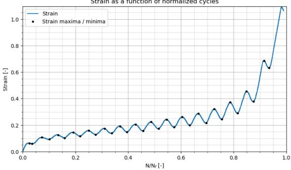
Strain as a function of normalized cycles
