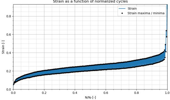
Strain as a function of normalized cycles
